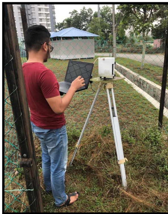
Figure 3.8: Getting the data from the HOBO rain gauge in KK2 in UMP Gambang
