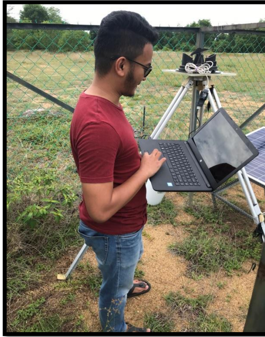
Figure 3.9: Getting the rainfall data from HOBO rain gauge in UMP Pekan campus
