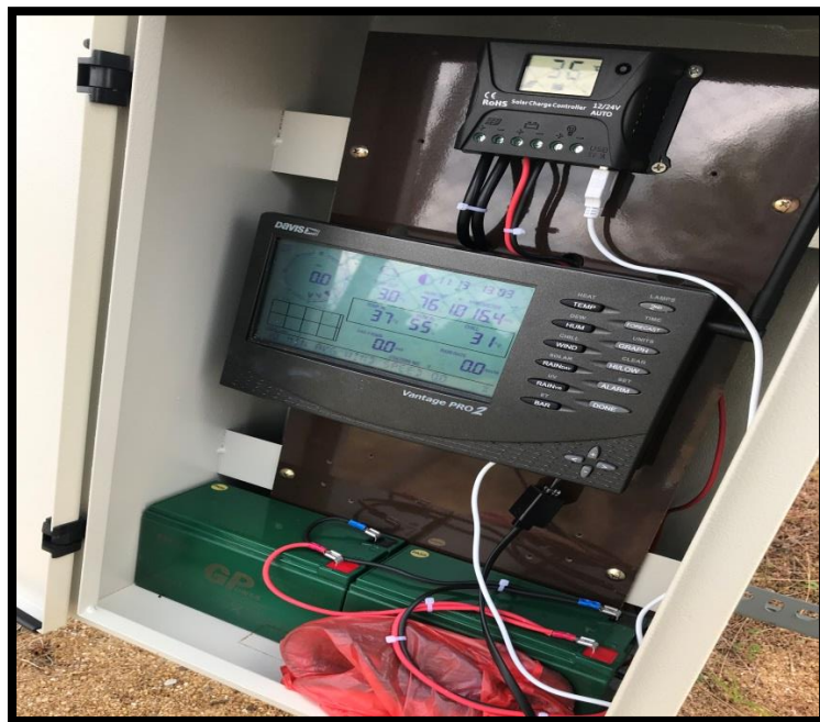
Figure 4.14: Weather station console successfully linked up with the solar panel and powered up by the solar panel
