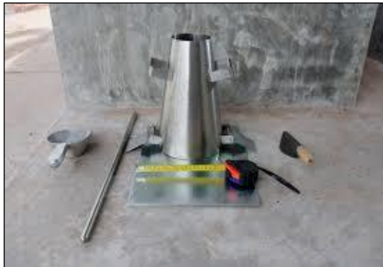
Figure 3. 7: Apparatus used in slump test
