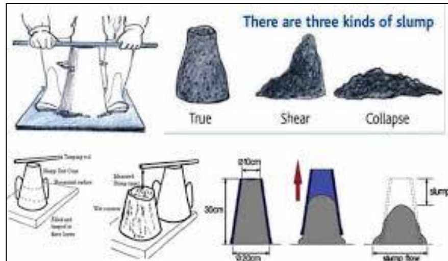
Figure 3. 6: Types of slump (BS 1881 Part 102: 1983)
