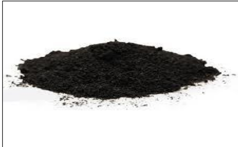
Figure 3. 4: Rubber Tire Waste Powder
