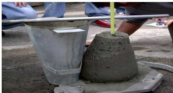
Figure 4. 1: Slump Test reading for sand replacement
