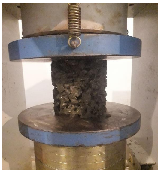
Figure 4.13 50% Granite - 50% steel slag
