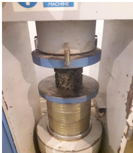
Figure 4.14 Compressive Strength for Cylindrical sample
