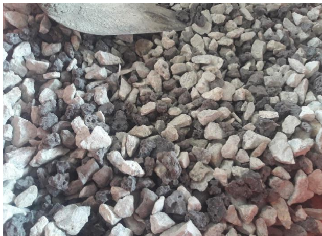
Figure 3.3 Steel Slag (dark colour) and Granite Aggregate
