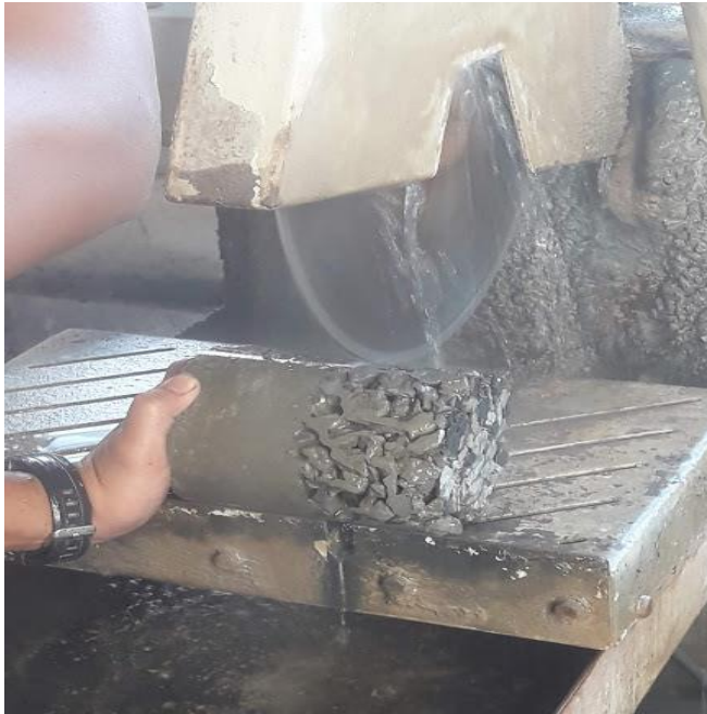
Figure 3.16 Take-off piece of the cylindrical sample
