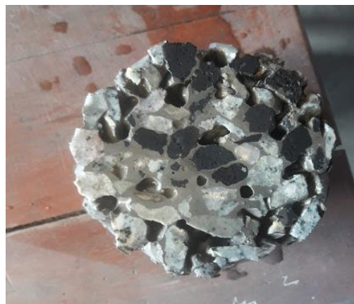
Figure 4.20 Appearance of Equal Amount of Steel Slag and Granite Aggregate in PC
