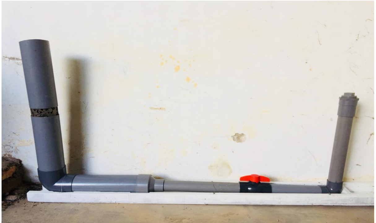
Figure 3.21 Falling Head test used for infiltration rate investigation
