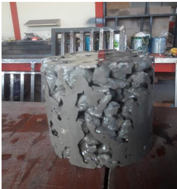
Figure 3.7 cylindrical samples of PC with steel slag.
