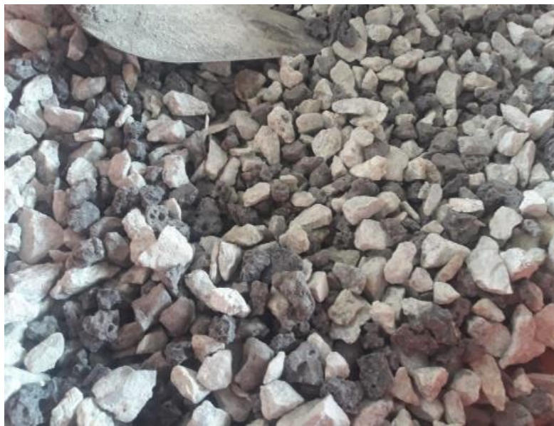
Figure 4.12 Steel Slag Mixed with Granite
