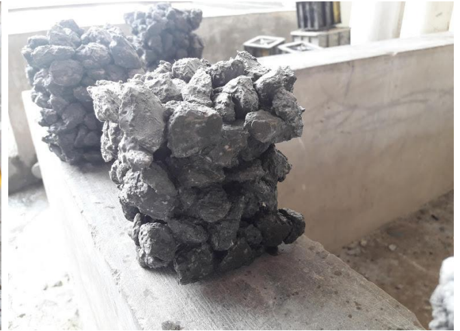
Figure 4.2 pervious concrete with Improper Vibration
