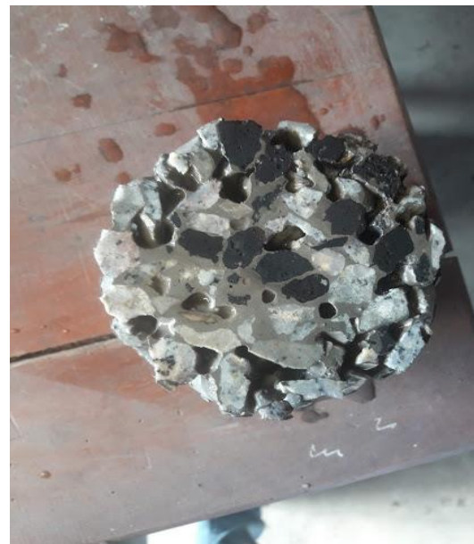
Figure 3.7 cylindrical samples of PC with steel slag.
