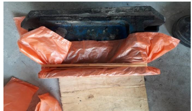
Figure 3.11 Rubber band binds the plastic bag
