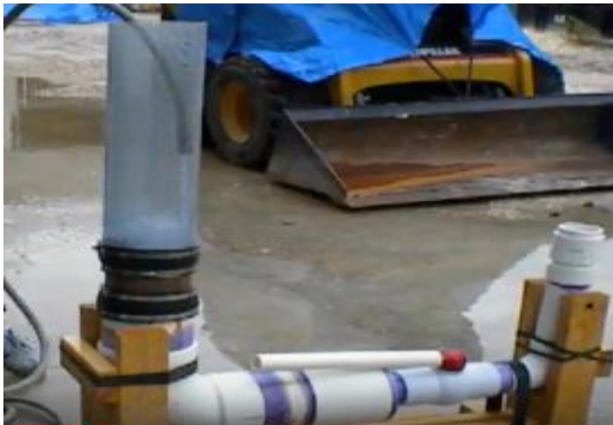
Figure 3.19 Permeability test (Falling Head Test)
