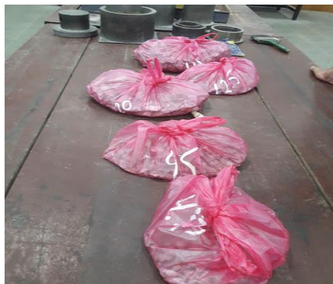
Figure 3.4 The 5 sizes of granite aggregate used
