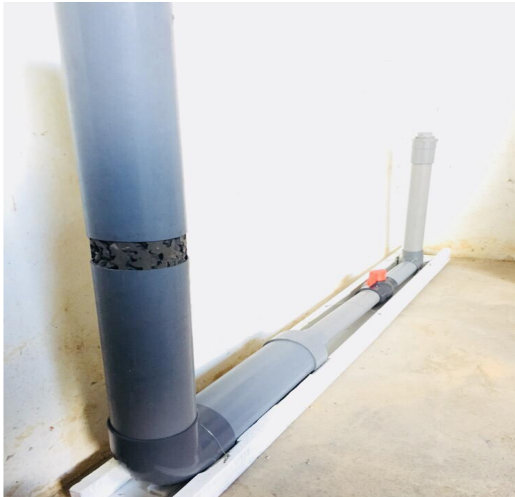
Figure 3.20 Sample is placed and were rubbed by silicon
