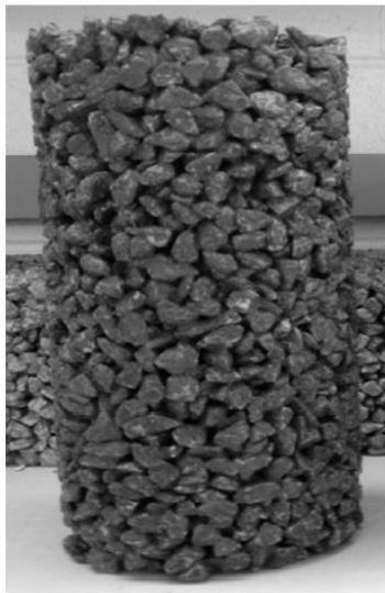
Figure 3.6 Cylindrical Sample of PC
