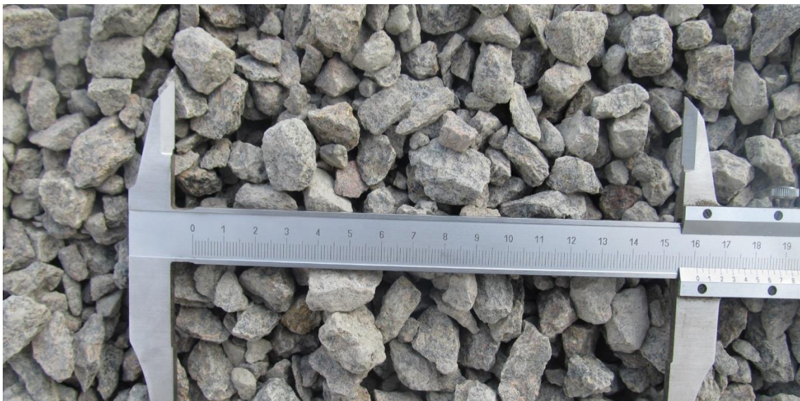
Figure 2.4 Granite Aggregate Size
