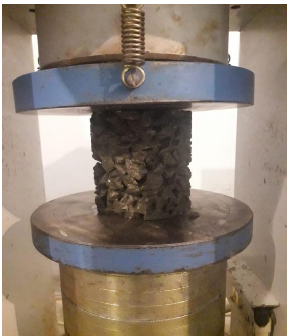
Figure 3.14 Compressive Strength Test
