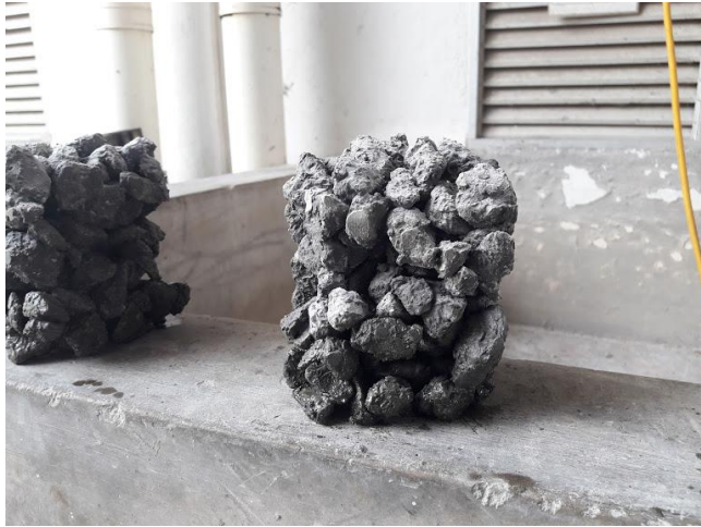
Figure 4.1 Zigzag Pervious Concrete Monolingual Aggregate Sample
