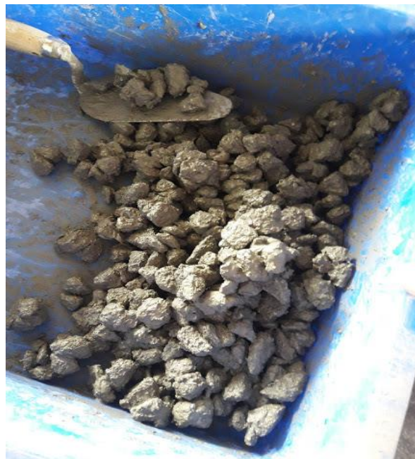
Figure 4.9 Low water content in the Mix 12
