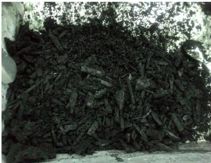
Figure 3.2: Production of sugarcane bagasse activated carbon in laboratory
