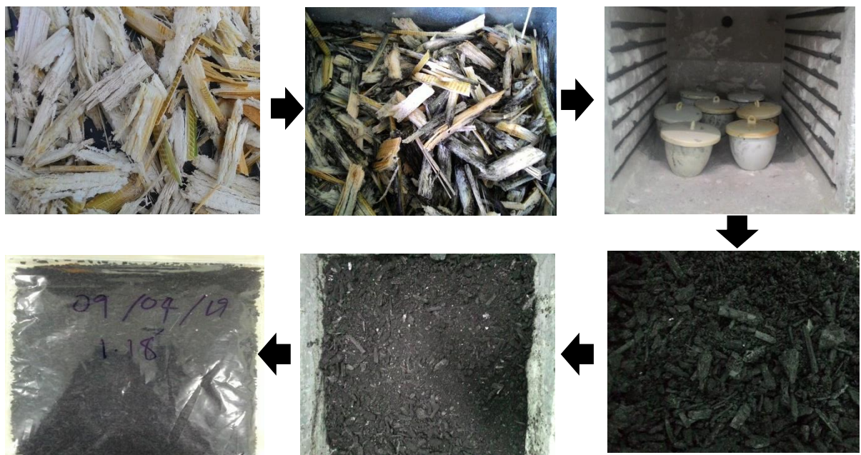
Figure 3.3: The process of sugarcane bagasse activated carbon
