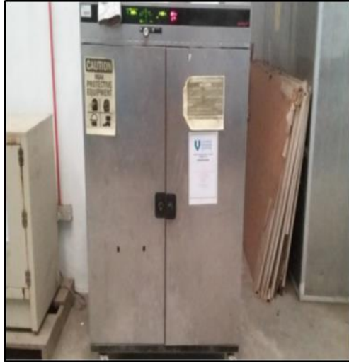
Figure 3.13: Oven to store the samples for water absorption test
