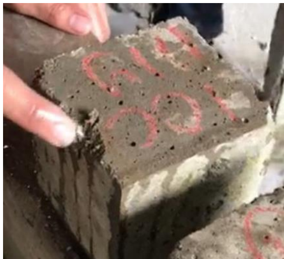
Figure 4.8: Cube sample when submerged in the water after few seconds
