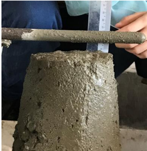
Figure 4.2: Slump value at 10% of sand replacement
