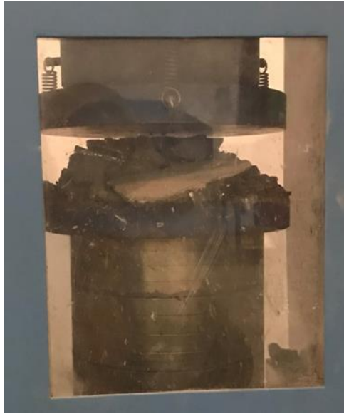
Figure 4.4: Cube sample with 5% of sludge after testing
