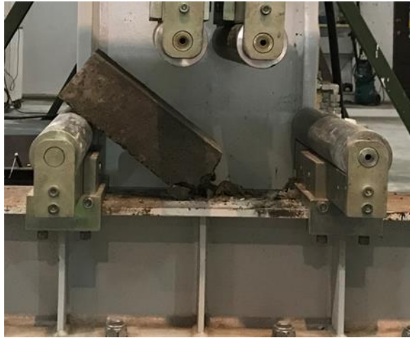
Figure 4.6: Prism sample after testing of 5% of sand replacement
