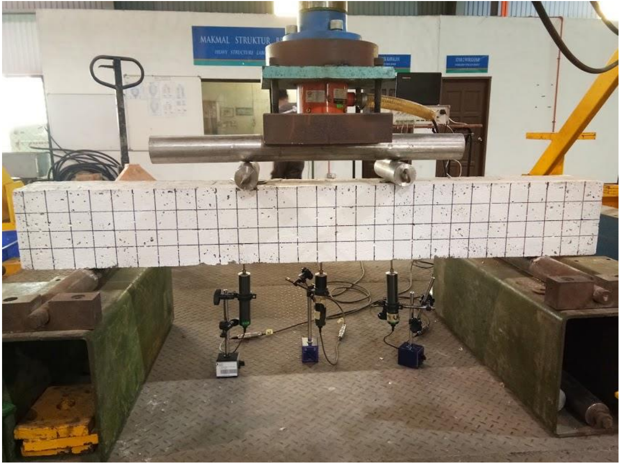
Figure 3.12: Setup of 4 points bending test.
