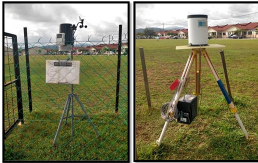
Figure 3.2: Example of tipping bucket rain gauge placed at Kolej Kediaman 2, Universiti Malaysia Pahang, Gambang.
