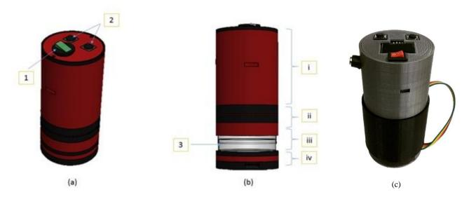
Fig. 1: The design of the developed portable soil Nitrogen sensor: (a) perspective view, (b) front view, and (c) proposed sensor after fabrication process: (1) switch, (2) push buttons, (3), petri dish, (i) main circuit compartment, (ii) NIR LEDs compartment, (iii) soil sample compartment, (iv) light sensing element circuit compartment.
