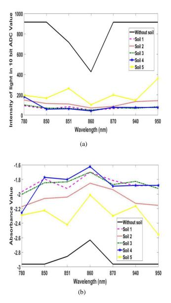
Fig. 3: The transmission intensity of NIR energies: (a) in 10 bit ADC Value, and (b) in the absorbance value.
