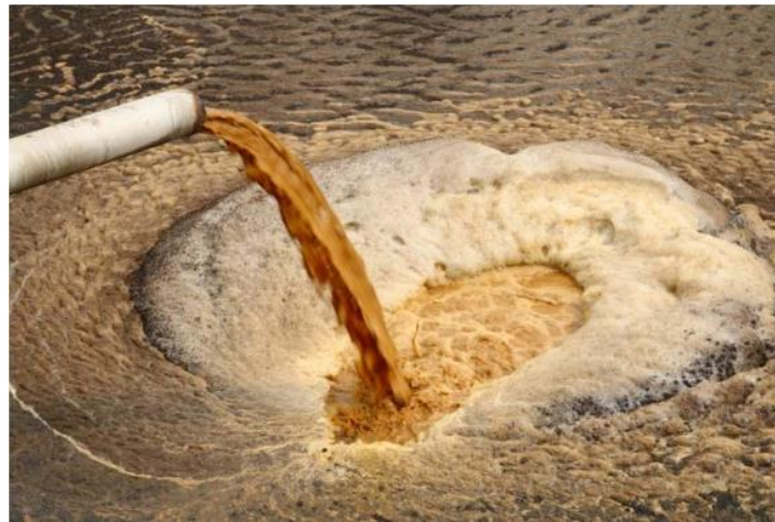
Figure 1.1 Discharge of palm oil mill effluent (POME) (image credit: Tan Kian Yong) (2015)
