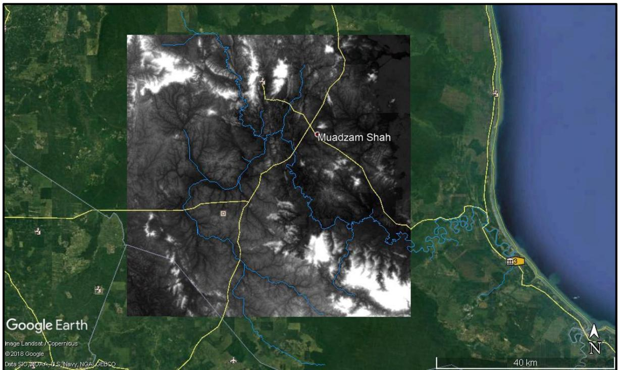
Figure 3.6 Projected SRTM DEM and river network in Google Earth
