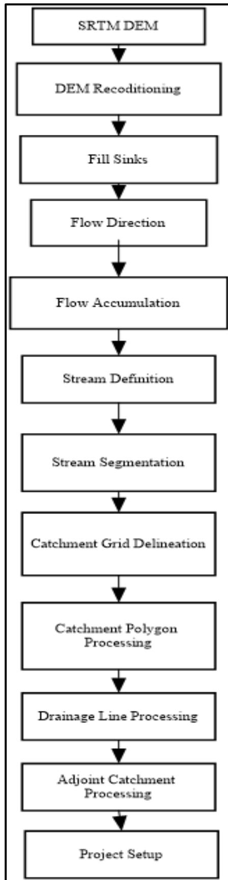
Figure 3.7 Flowchart of Method of River Basin Delineation
