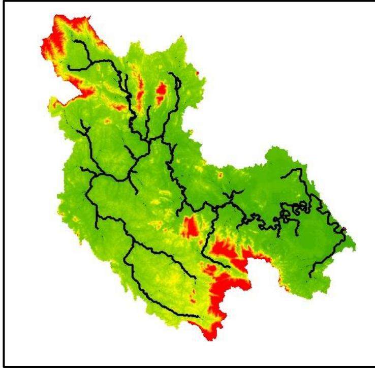
Figure 4.3 The delineated river network (30m resolution)
