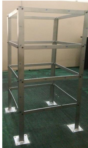
Figure 1. Frame Structure with bolted joints
