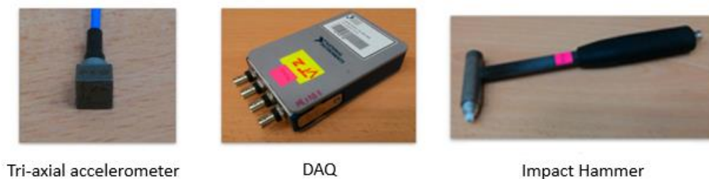
Figure 3. Impact hammer equipment
