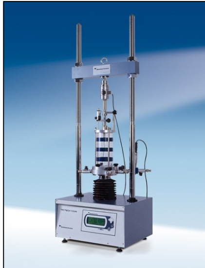
Figure 3.10: Unconfined Unconsolidated devices
