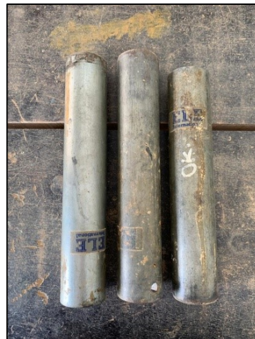
Figure 3.8: Shelby tube sampler used in the study
