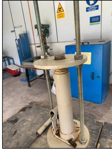
Figure 3.9: Soil extruder used to extrude soil sample
