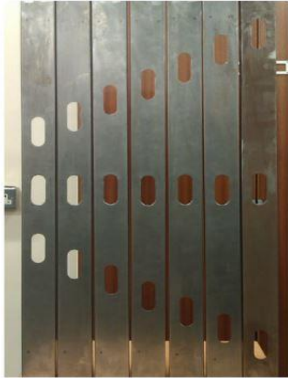
Figure 1.4 Example of cold-formed steel with different position of openings Source: Kulatunga and Macdonald (2013)
