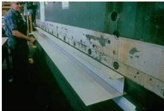
Figure 2.4 Press braking method
