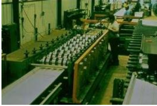
Figure 2.3 Cold-roll forming method
