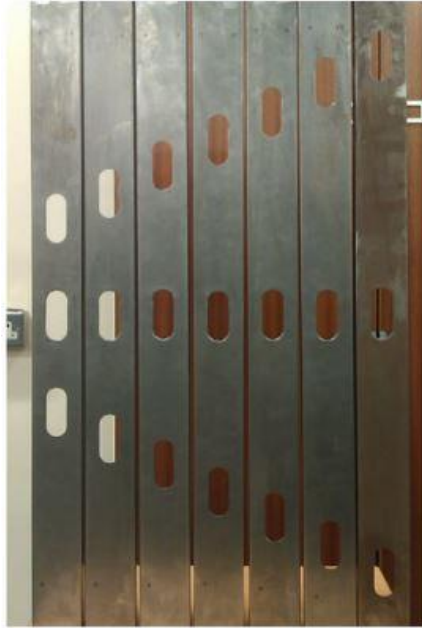
Figure 3.15 Series of cold-formed C-section with various position of perforation
