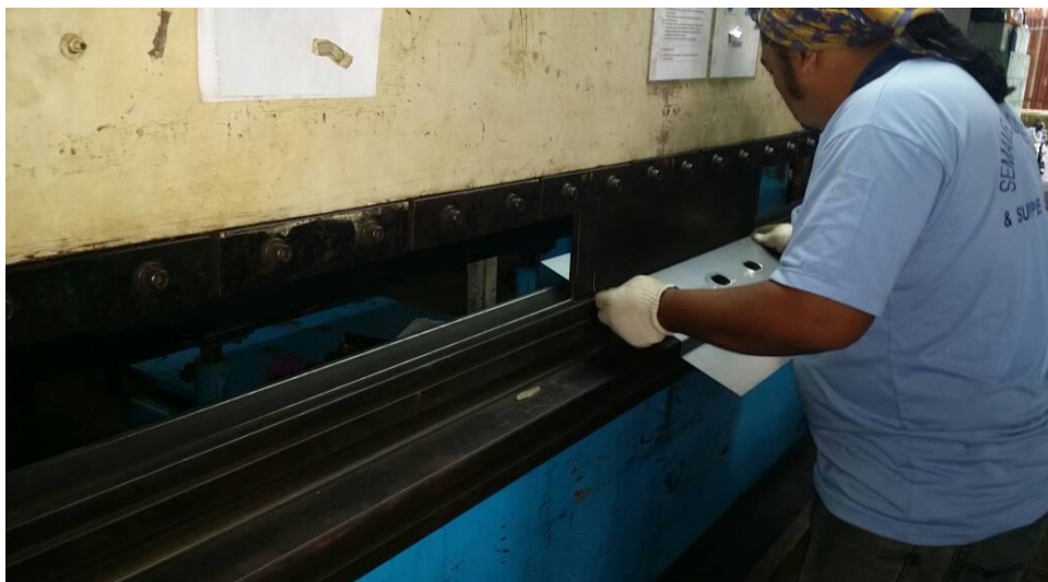
Figure 3.6 Process of shaping the cold rolled sheet
