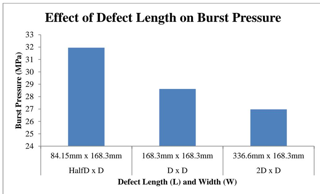
Figure 4.4 Result of defect length on burst pressure
