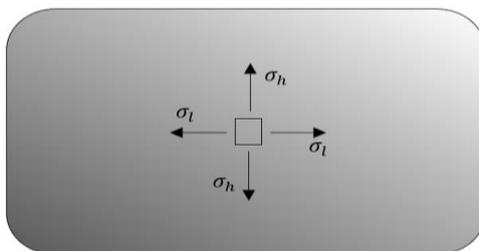
Figure 2.4 Direction of hoop and longitudianl stress
