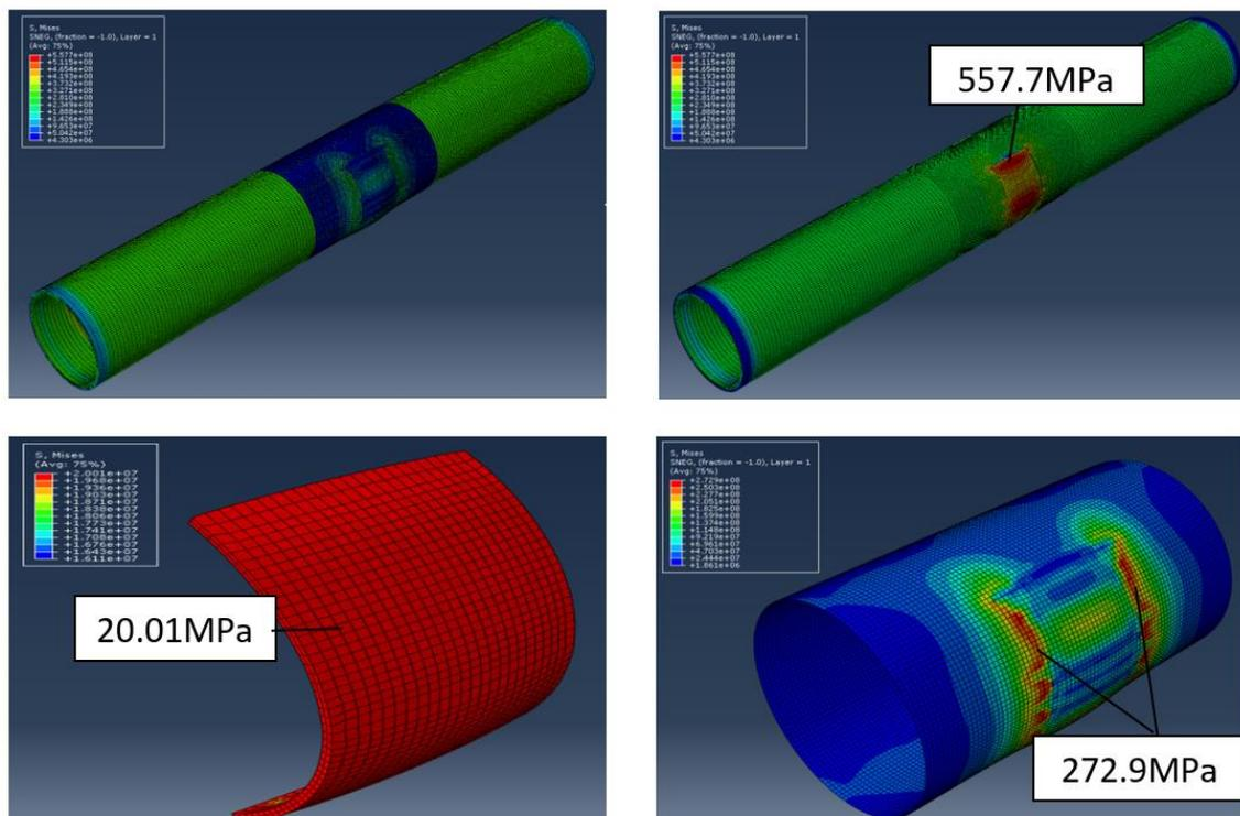
Figure 4.1 Stress Contour Plot for the *Half D* composite repaired-pipe model
