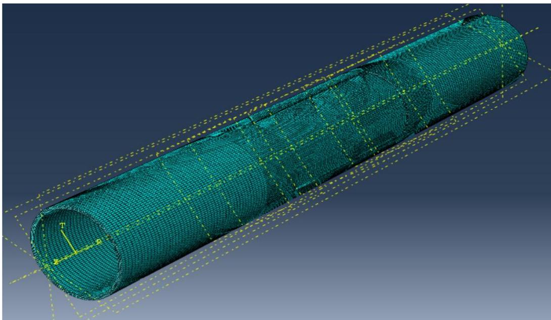
Figure 3.6 Example of a meshed defective pipe
