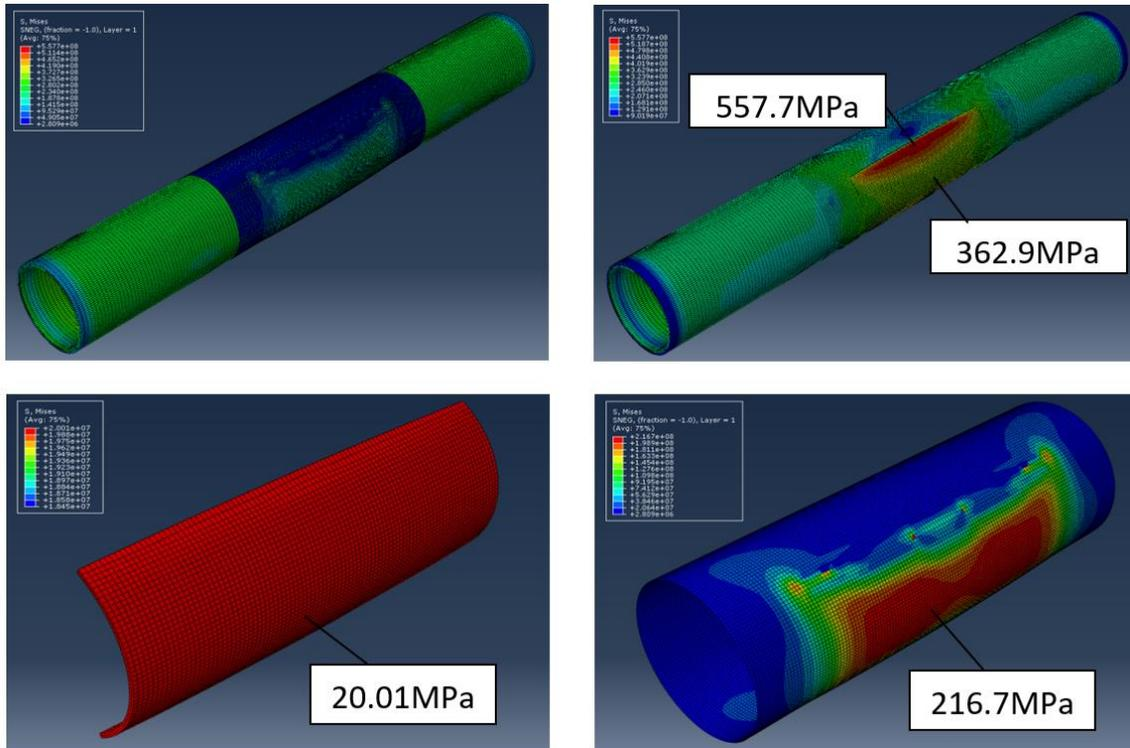
Figure 4.3 Stress Contour Plot for the 2D composite repaired-pipe model
