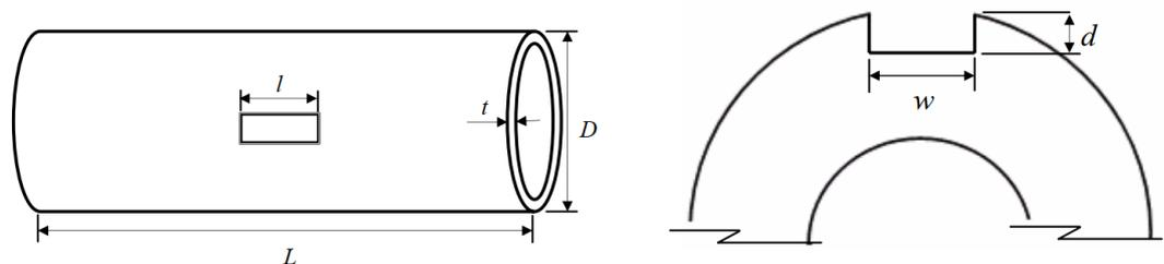
Figure 2.1 Defect Geometries in Schematic Defective Pipelines
