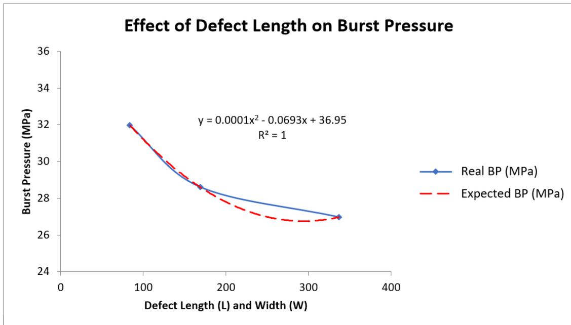
Figure 4.5 Effect of defect length on burst pressure
