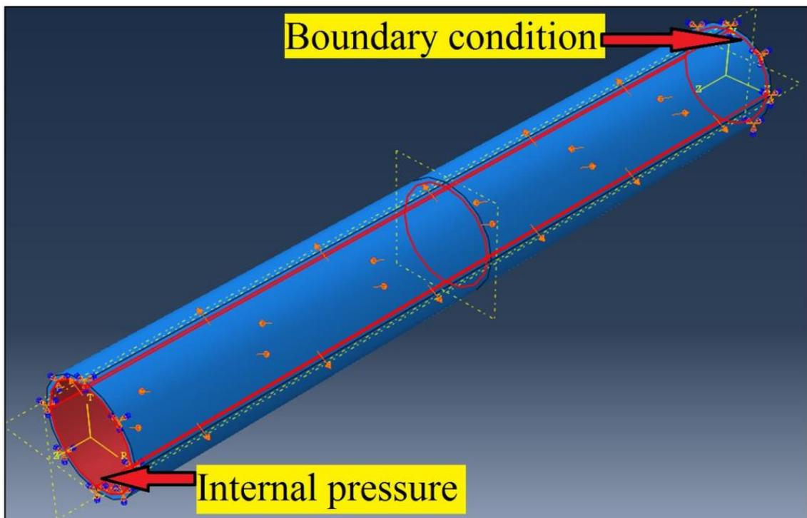
Figure 3.4 Internal pressure and boundary condition
