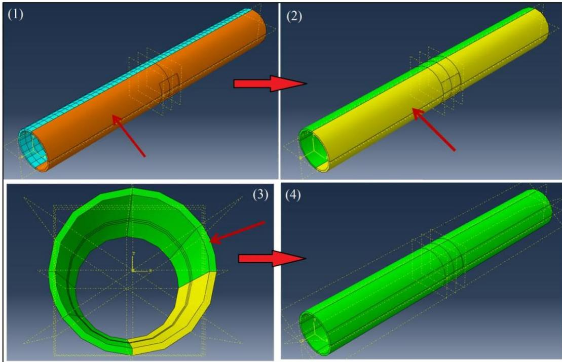
Figure 3.5 Process in achieving structural mesh
