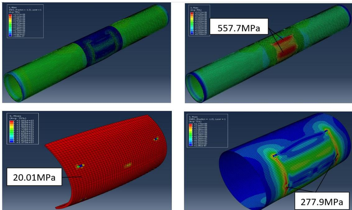
Figure 4.2 Stress Contour Plot for the *D* composite repaired-pipe model
