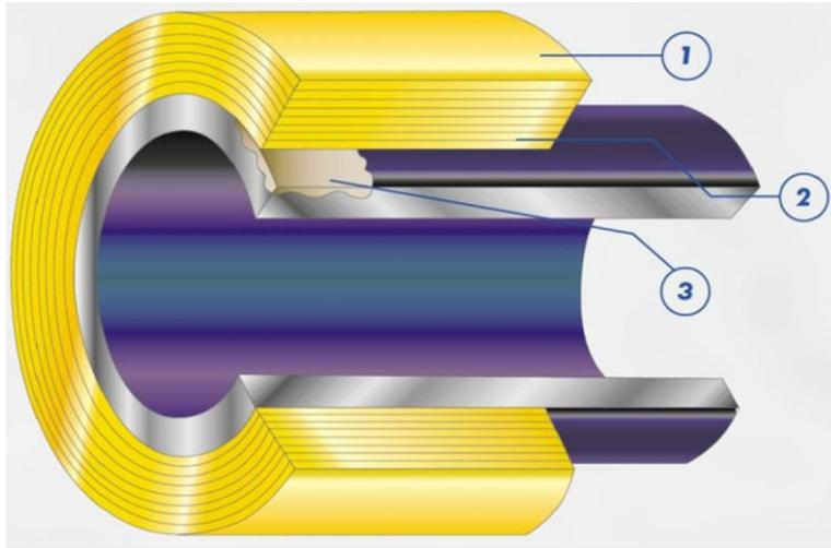
Figure 2.3 Clock Spring ® FRP composite repair system with FRP composite (1), Interlayer adhesive (2), and Infill material (3)
