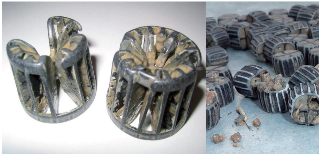
Figure 7. Shown biofilm growth at the inside layer of a commercial carrier [65].
