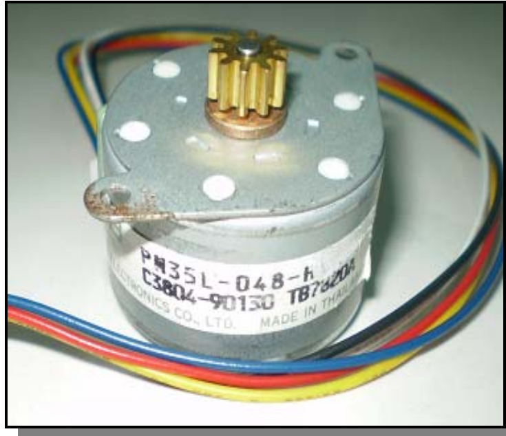
Figure 3.12: 5-wire Unipolar Stepper Motor Connection
