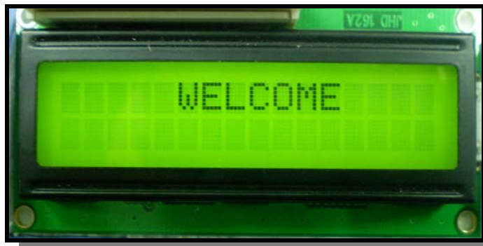
Figure 2.7: 2 lines (8 character) JHD162A LCD display
