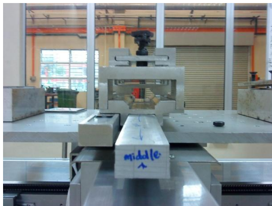
Figure 4.7: Back view of the MIG welding jigs when mounted on the welding table.
