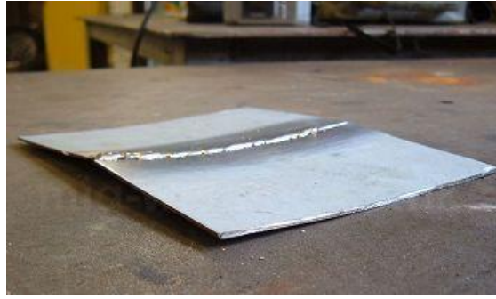
Figure 2.4: Distortion in sheet metal due to MIG welding (MIG Welding – the DIY Guide)
