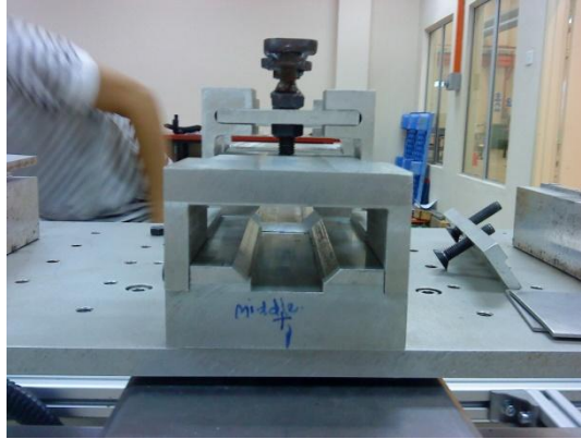
Figure 4.5: Front view of the MIG welding jigs when mounted on the welding table.
