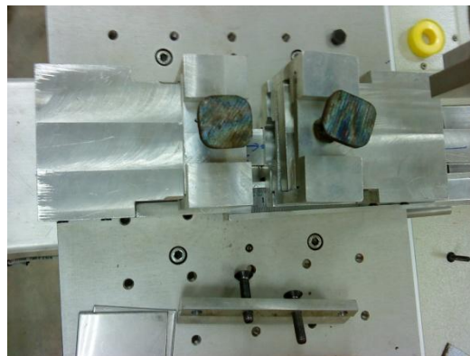
Figure 4.4: Top view of the MIG welding jigs when mounted on the welding table.
