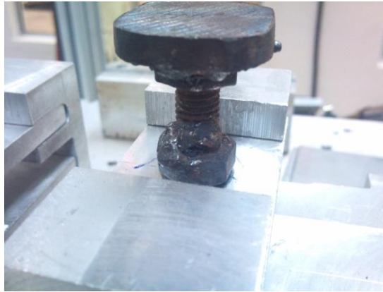
Figure 4.15: Defect due to welding.
