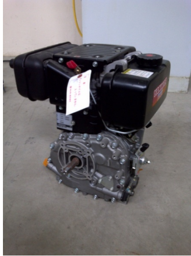
Figure 2.1: A 4 Stroke Diesel Engine
