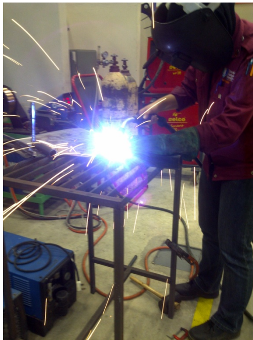
Figure 3.5: Joining the part for the engine test platform
