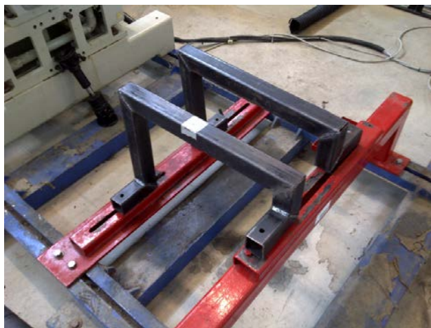
Figure 3.7: Complete engine test platform with the existing stand
