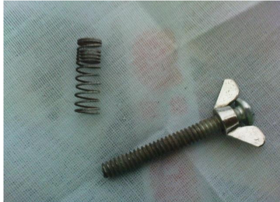
Figure 3.5: screw and spring as lock part
