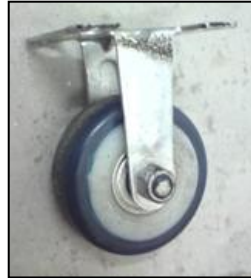
Figure 4.19: Non-lockable castor without bearing
