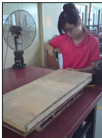
Figure 3.12: Material joining (Nailing)
