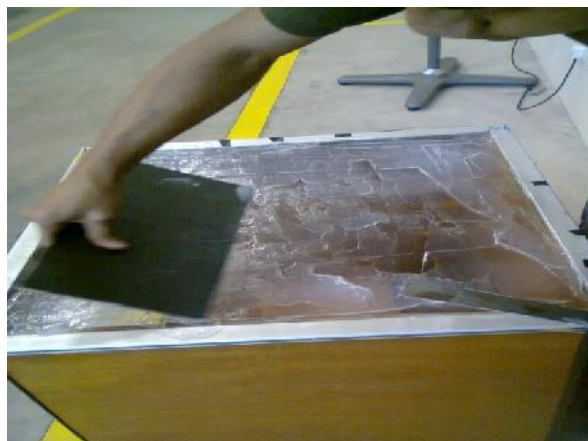
Figure 3.17: Pouring silicone onto acrylic surface
