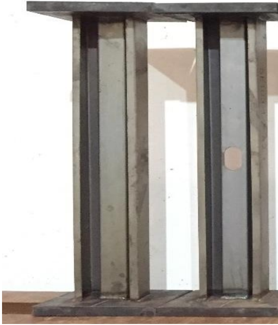
Figure 1.3 Examples of the specimen with an opening and without opening
