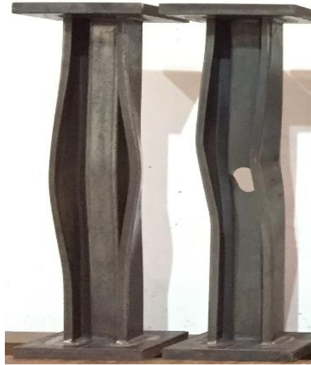
Figure 4.8 Specimen SE103-2.0-A1 (left) and SE103-2.0-A2 (right) AFTER testing
