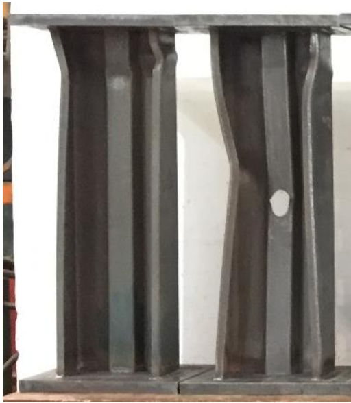
Figure 4.10 Specimen SE203-2.0-A1 (left) and SE203-2.0-A2 (right) AFTER testing
