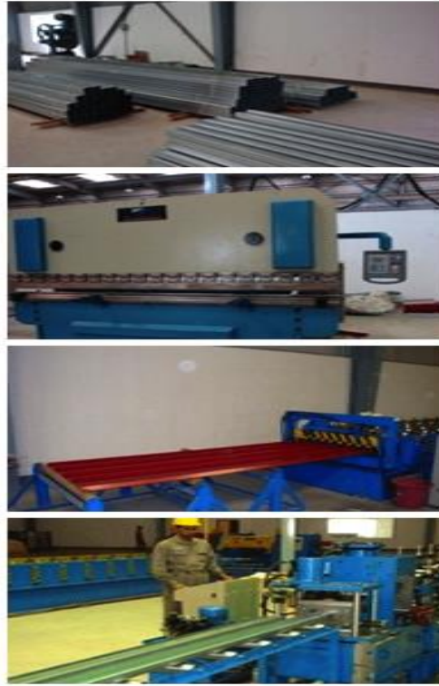
Figure 3.2 Process of fabrication of cold-formed steel
