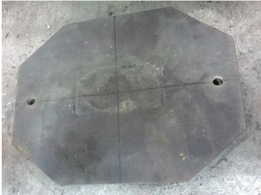
Figure 3.5 Bearing plate that welded at the top and bottom of the specimen
