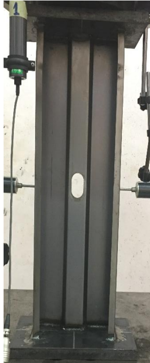
Figure 3.6 Position of an opening is constant at the middle of the specimen
