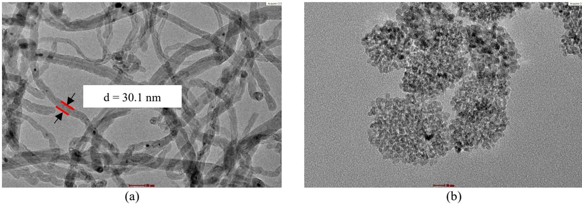
**Figure 1.** TEM images of (a) MWCNTs-doped 10 wt% graphene nanoparticles and (b) TiO<sub>2</sub> nanoparticles.
