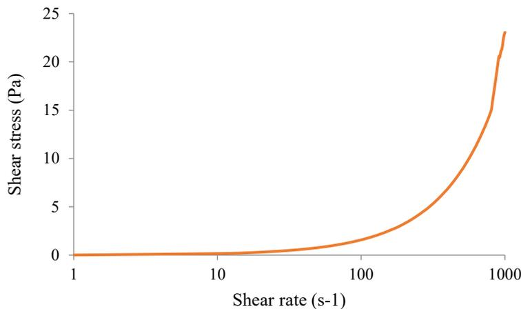
**Figure 5:** Shear stress vs shear strain curves for TiO<sub>2</sub>-CNTs nanofluid with a concentration of 0.02%.
