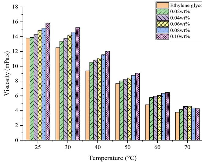
**Figure 4.** Viscosity of TiO<sub>2</sub>-CNTs nanofluids as a function of temperature at different volume fractions, compared to base fluid (ethylene glycol).
