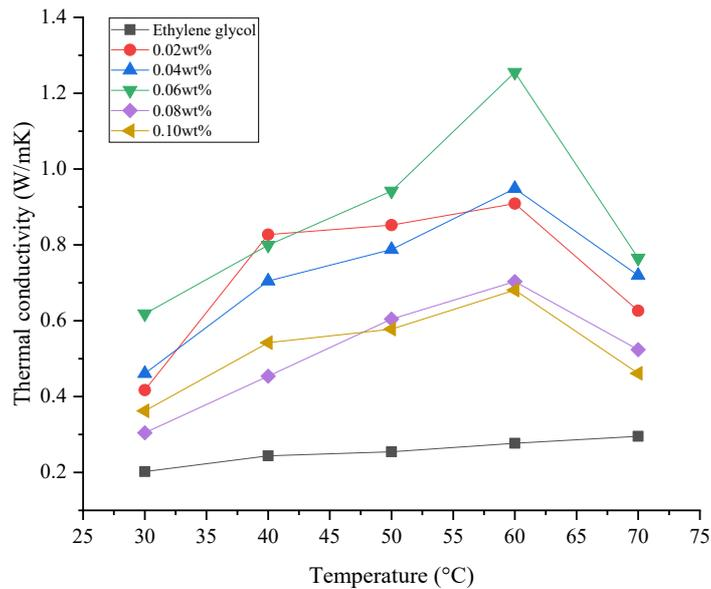
**Figure 3.** Thermal conductivity of TiO<sub>2</sub>-CNTs hybrid nanofluids as a function of temperature and volume fractions, compared to base fluid (ethylene glycol).
