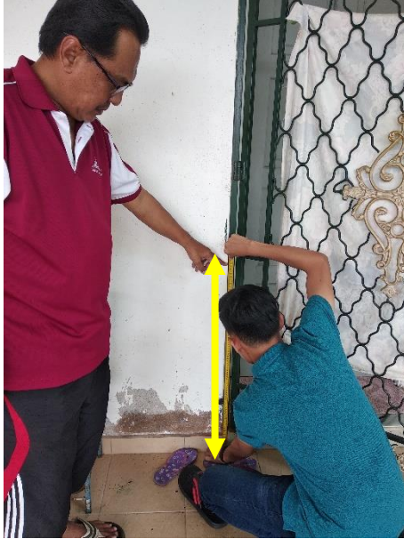
Location: Permatang Badak Baru Flood depth: 0.8 m
