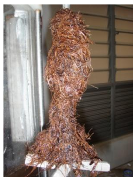
Figure 5: Fiber stacked at centre of impeller shaft
