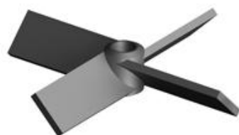
Figure2: Pitch blade turbine (PBT) with impeller diameter, D = 0.4T
