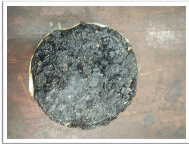
Figure 3.8: Sample before abrasion test
