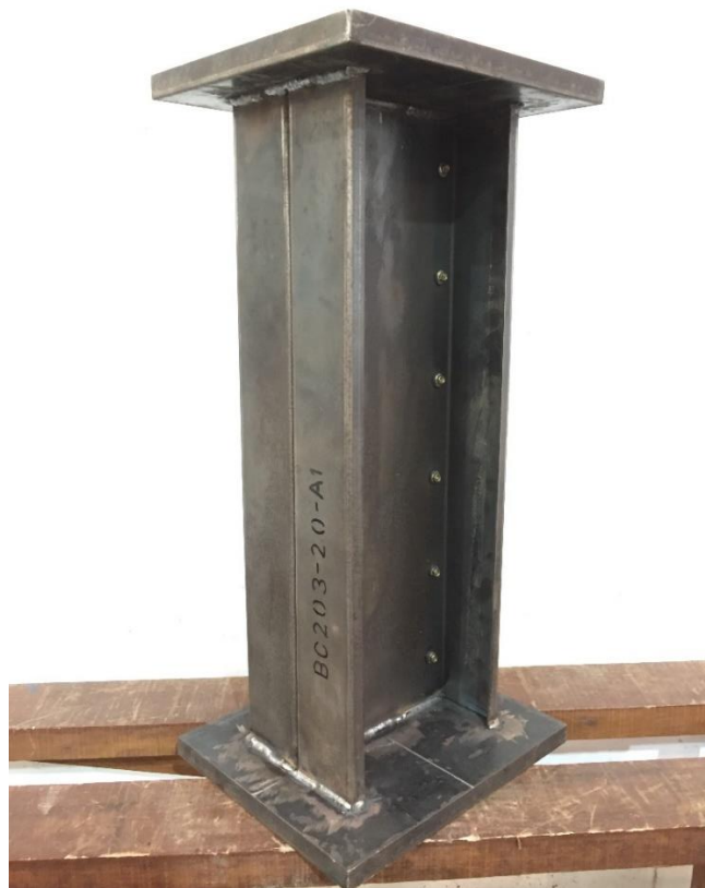
Figure 3.15 Specimen welded at top and bottom support
