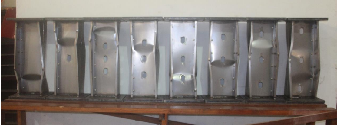
Figure 4.11 Eight specimens for BC 203-1.2 after testing
