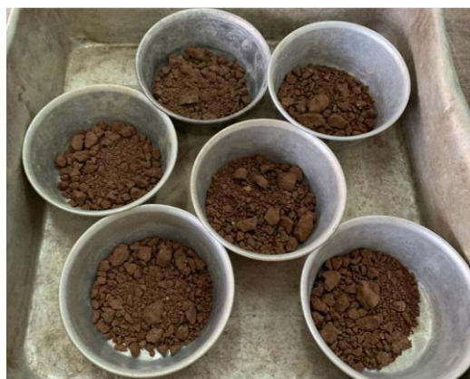
Figure 3.6 Cooling dry soil
