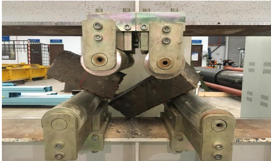
Figure 4.10 Failure mode of plain concrete beam
