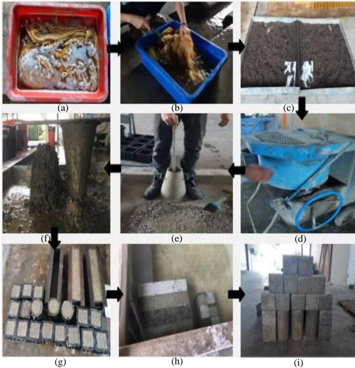
Figure 3.2 Procedure of laboratory work. (a) Alkaline treatment of the extracted fibre. (b) Clean the fibre after soaking to remove NaOH. (c) Air-dry the OPS after soaking in water for 24 hours (d) After all materials are prepared, use the concrete mixer to mix all the materials. (e) Construct the slump test before pouring fresh concrete in mould. (f) Obtain the slump value for true slump. (g) Pour the fresh concrete mix in moulds. (h) After 24 hours, unmoould the specimens and cure them in water.
