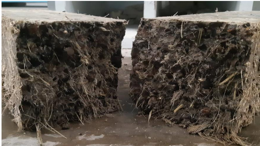
Figure 4.12 PALF bridging inside the concrete
