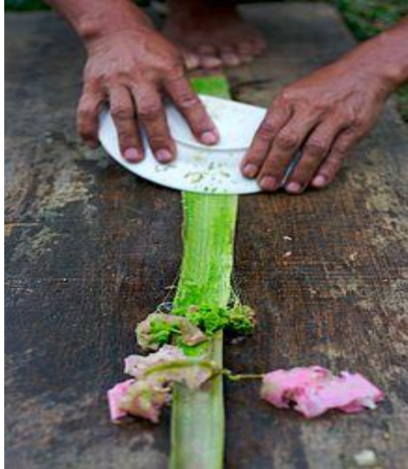
Figure 2.8 Manual extraction of PALF
