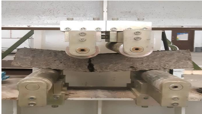
Figure 4.11 Failure mode of 2.0% PALF reinforced concrete beam
