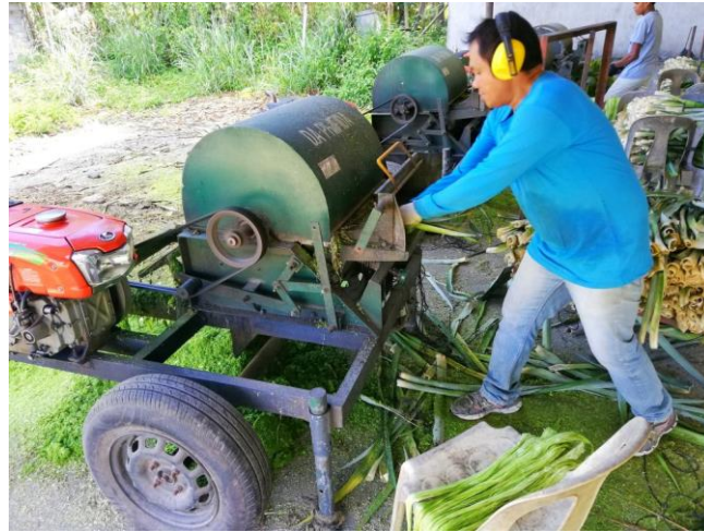
Figure 2.9 Mechanical extraction of PALF
