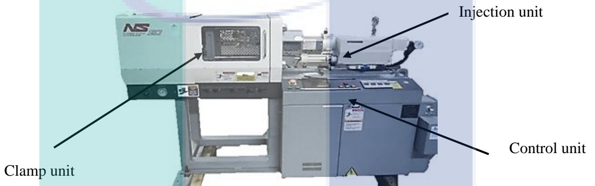
Figure 3.10 NISSEI 20-tonne injection moulding machine components
