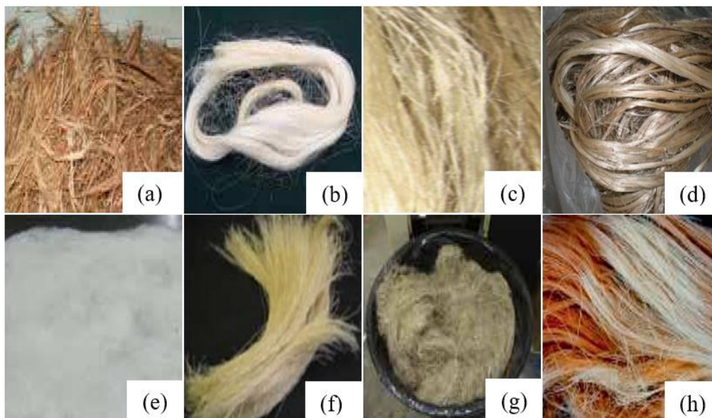
Figure 3. Natural fibers. (a) Coir fiber [12], (b) Sisal fiber [12], (c) Unidirectional jute fiber [2], (d) Kenaf fiber [13], (e) Cotton fiber [12], (f) Bamboo fiber [14], (g) Hemp fiber [12], (h) Pineapple fiber [15]
