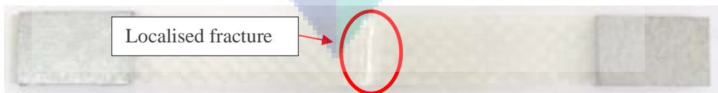
Figure 4.3 Tensile tested for GFRP specimen
