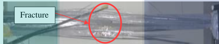
Figure 4.7 Tensile tested for specimen UD-CFP specimen
