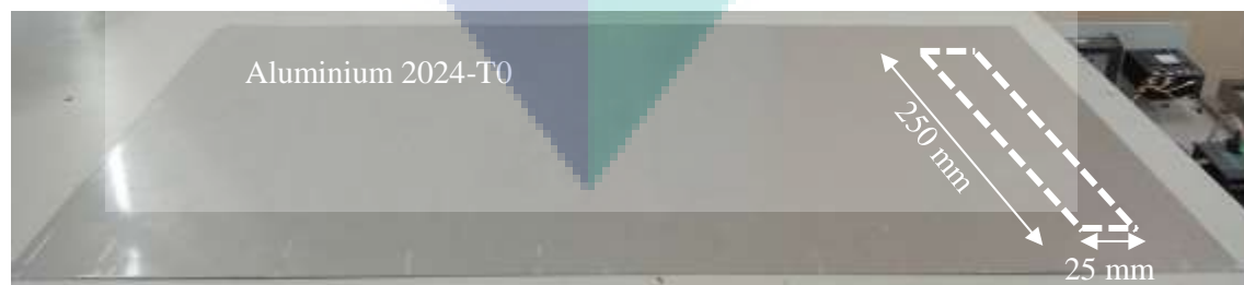
Figure 3.4 A plate of aluminium before cutting to size of 250 mm by 25 mm.
