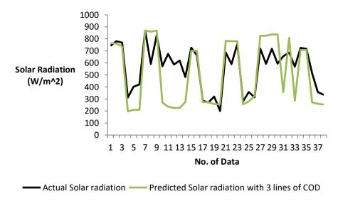
**Fig. 14.** Actual solar radiation and prediction results for 5 minute in advanced with COD as input
