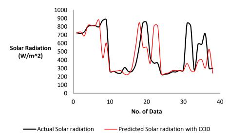
**Fig. 10.** Actual solar radiation and prediction results for 1 minute in advanced with COD as input
