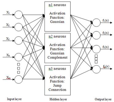
Fig. 6. Artificial neural network configuration
