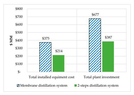
**Figure 5.** Comparison of capital investment of FW fermentation with membrane distillation and two-step distillation system for the separation process.
