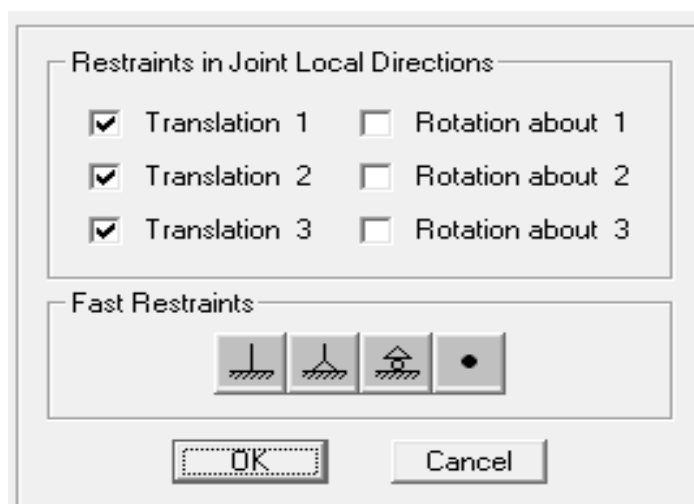
Figure 3.12 The preferred choice of joint restraint.
