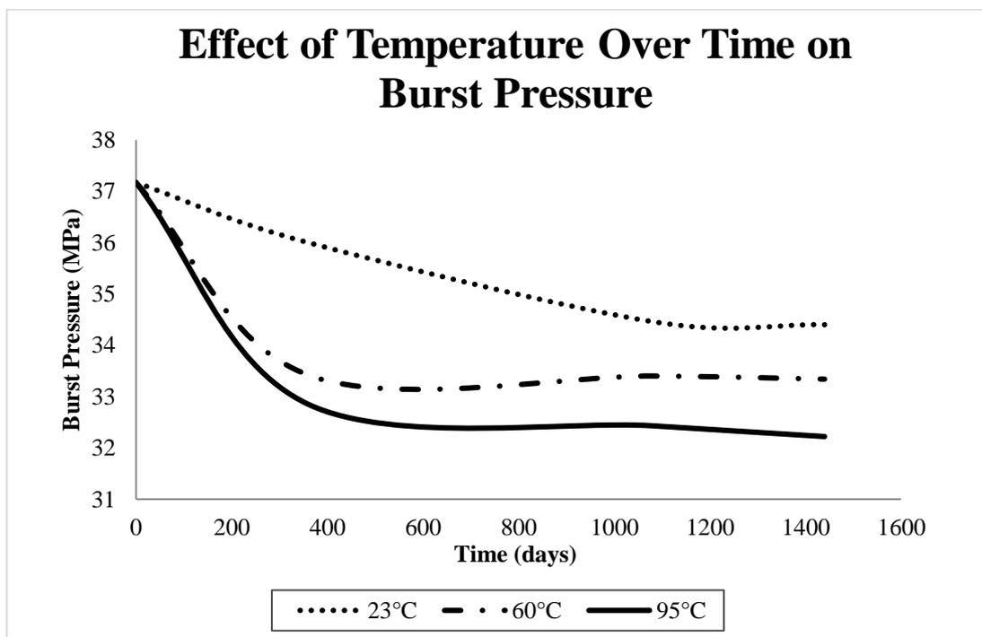
Figure 4.8 Effect of temperature over time when subjected to 23°C, 60°C, and 95°C
