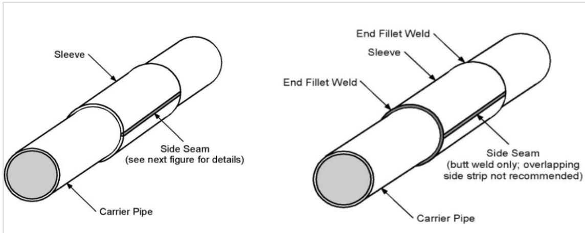
Figure 2.1 Type A sleeve (left) and Type B sleeve (right)
