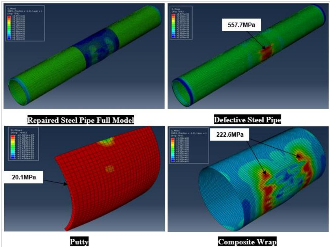
Figure 4.7 Contour stress plot of repaired pipe subjected to 95°C at 1440-days
