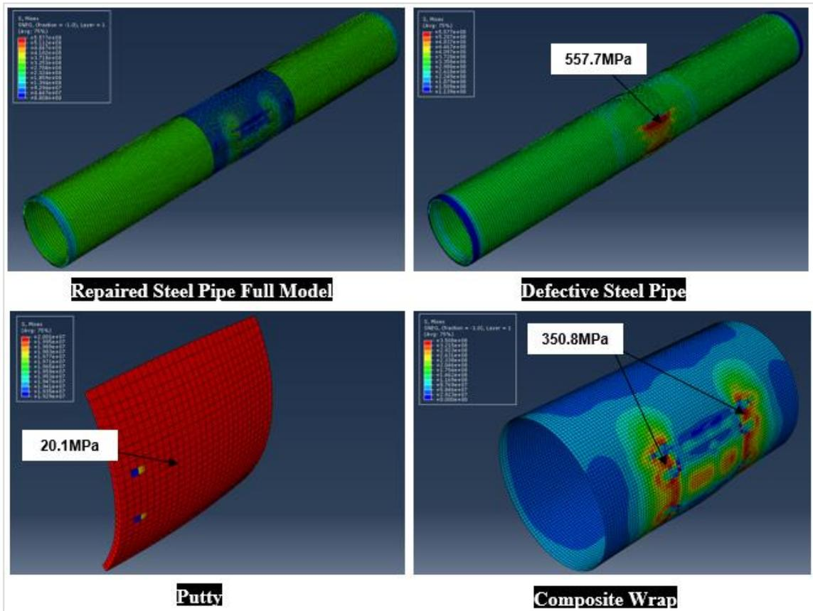
Figure 4.4 Contour stress plot of repaired pipe subjected to 60°C at 360-days
