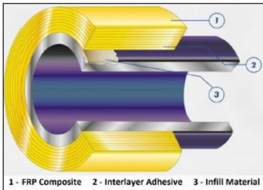
Figure 2.5 Clock Spring® components
