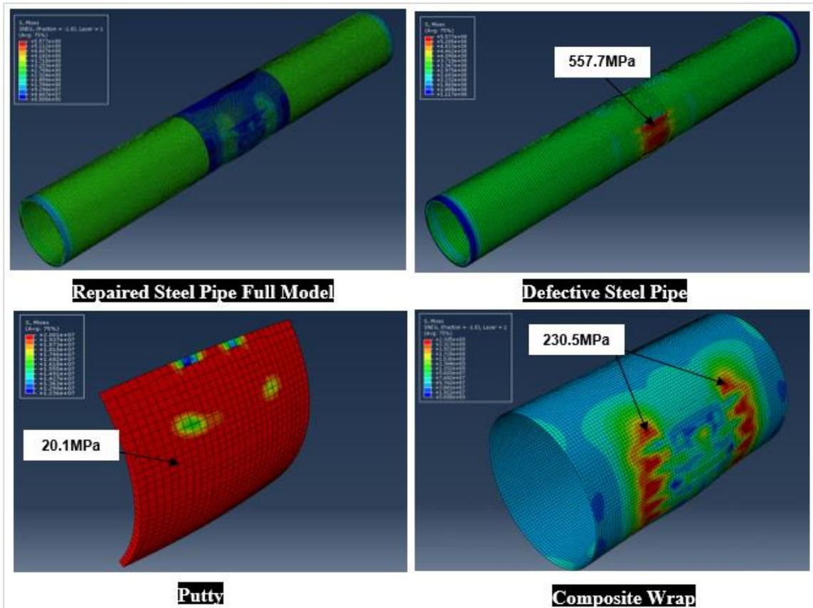
Figure 4.6 Contour stress plot of repaired pipe subjected to 95°C at 1080-days
