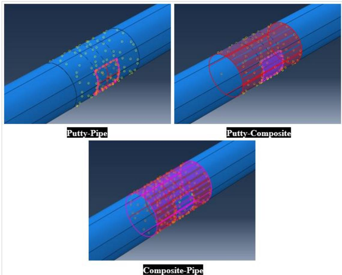
Figure 3.3 Bonding between putty-pipe, putty-composite, and composite-steel
