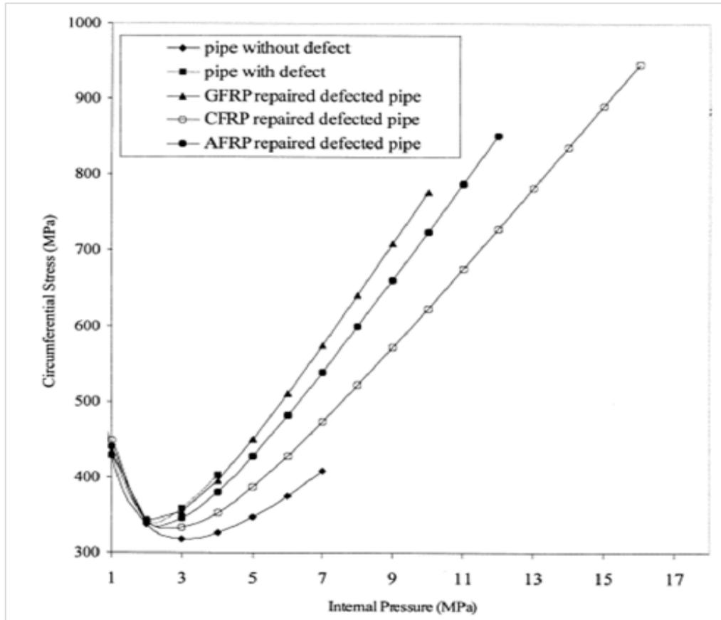
Figure 2.7 Comparison between circumferential stress and internal pressure in the pipe without defect, pipe with defect, and repaired damaged pipes
