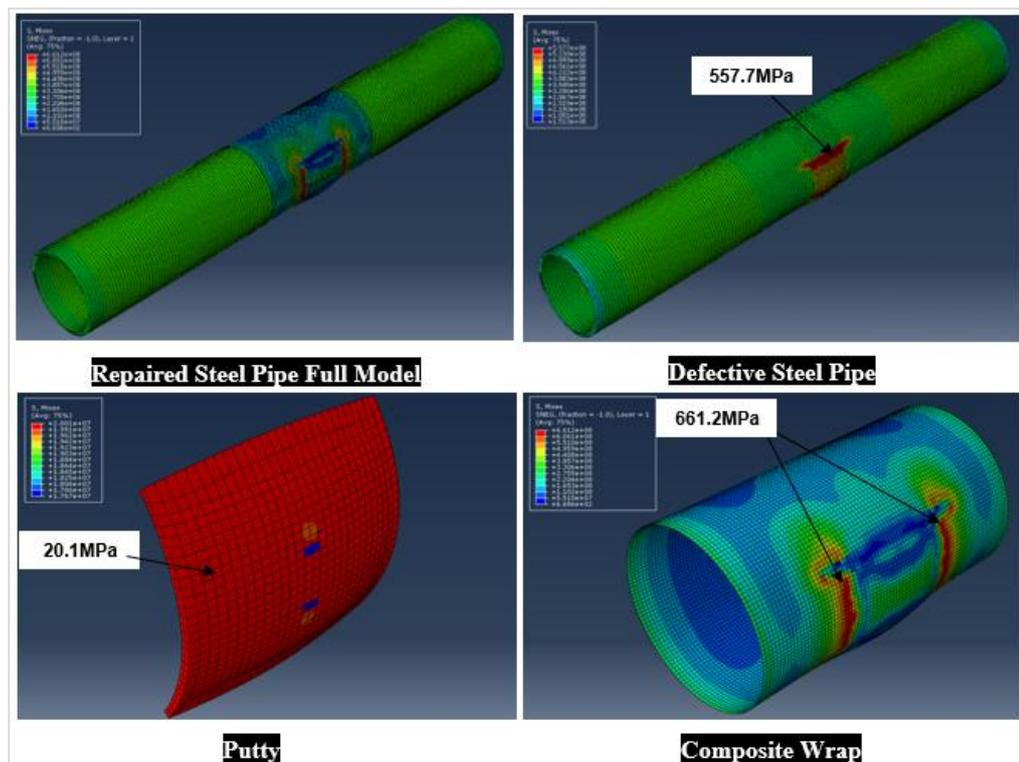
Figure 4.3 Contour stress plot of repaired pipe subjected to 23°C at 1440-days
