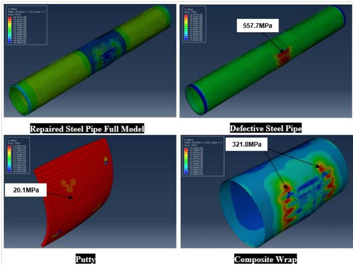
Figure 4.5 Contour stress plot of repaired pipe subjected to 60°C at 1440-days
