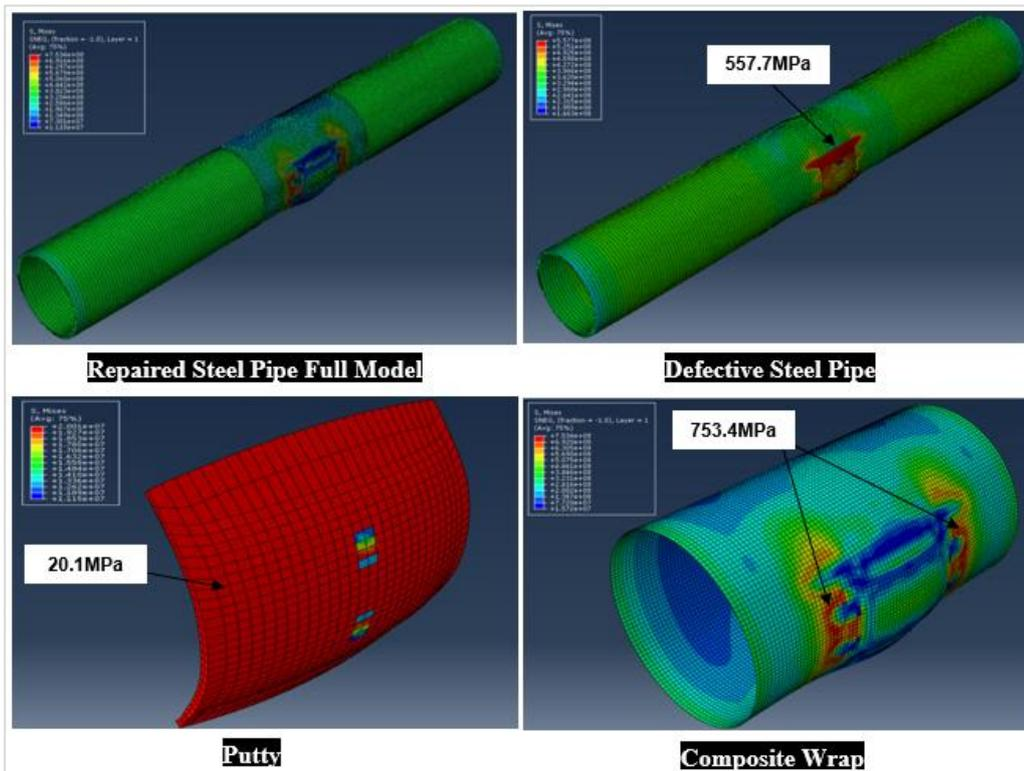
Figure 4.2 Contour stress plot for initial material pipe model (0-days)
