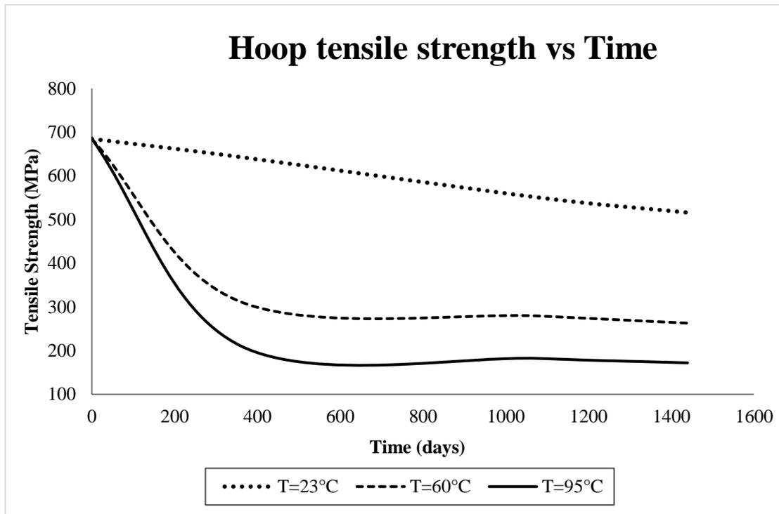
Figure 4.1 Hoop tensile strength of E-glass/Vinylester composite over time when subjected to 23°C, 60°C, and 95°C
