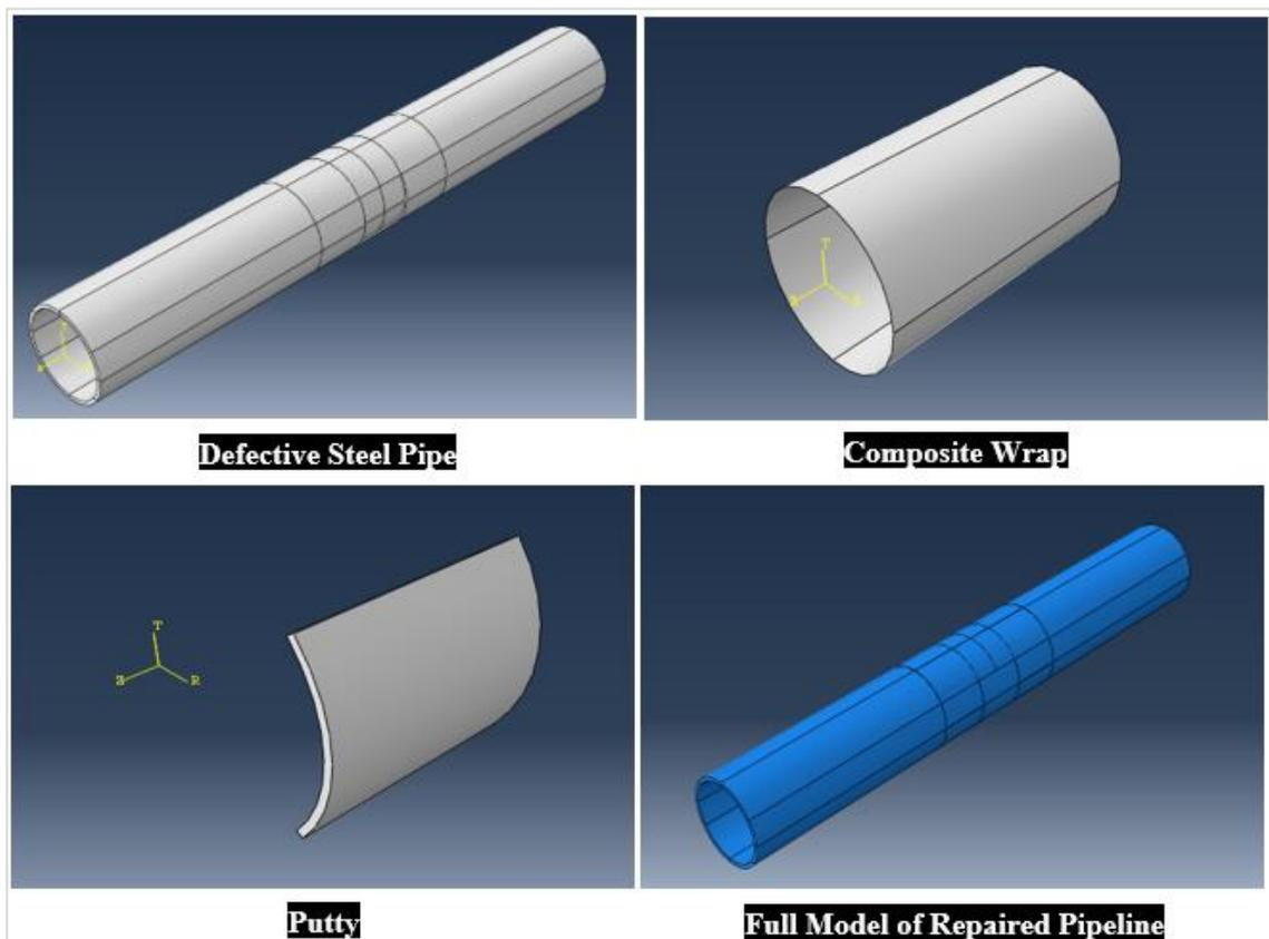
Figure 3.2 Geometry of defective steel pipe, composite, putty and integrated structure (full model-composite repaired steel pipe)
