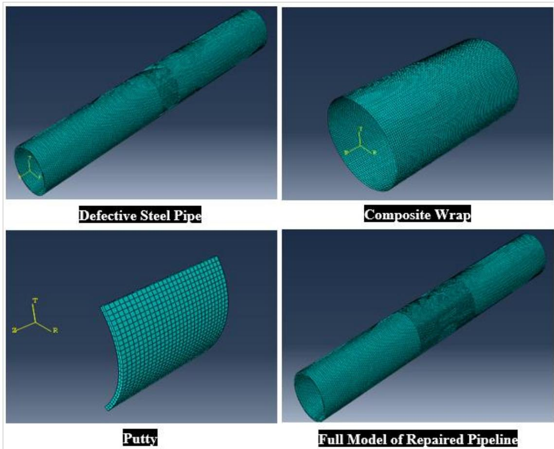
Figure 3.4 Meshed model of defective steel pipe, composite wrap, putty, and full model repaired pipe
