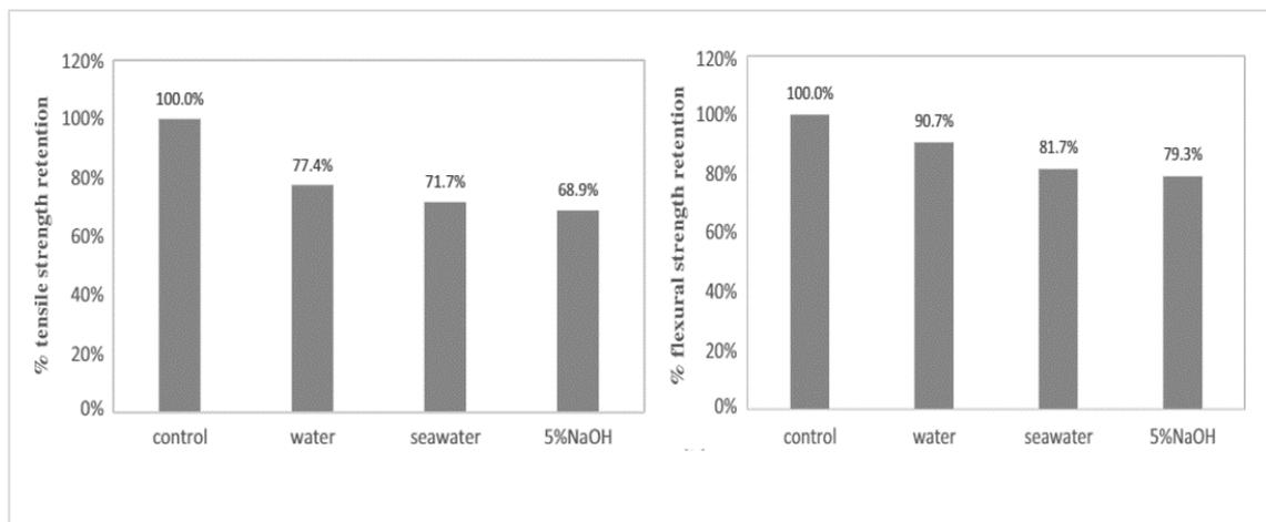
Figure 2.9 Percentage of tensile strength (left) and flexural strength (right) retained for flax fabric/epoxy composites after 365 days immersion
