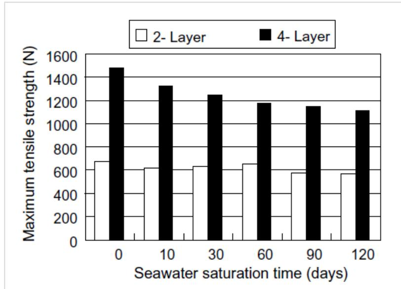
Figure 2.8 Tensile strength of seawater treated samples
