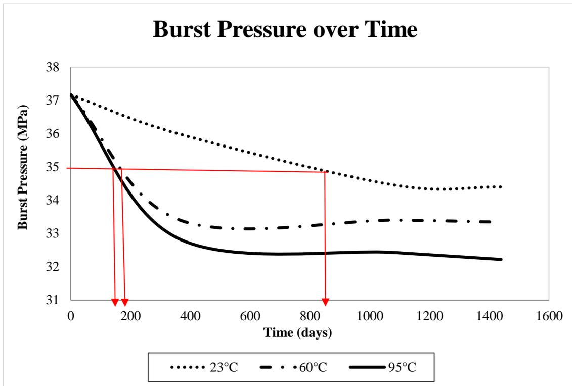
Figure 4.9 Prediction residual service lifetime of repaired pipe
