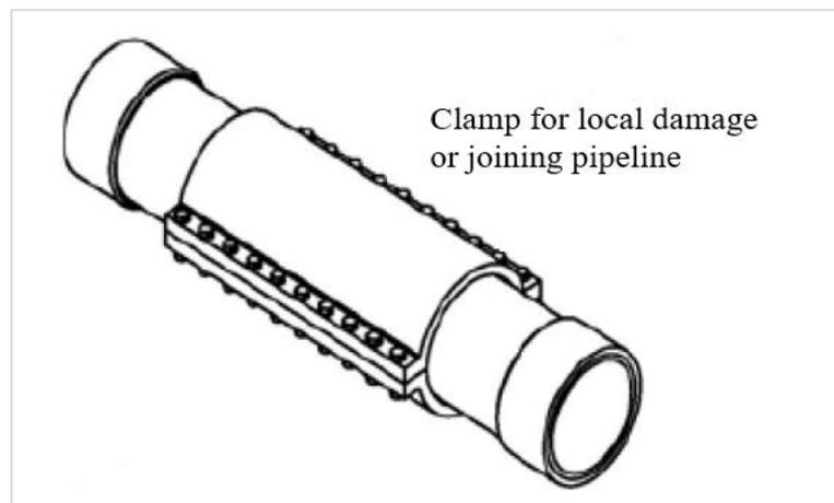
Figure 2.2 Typical mechanical bolt-on clamp
