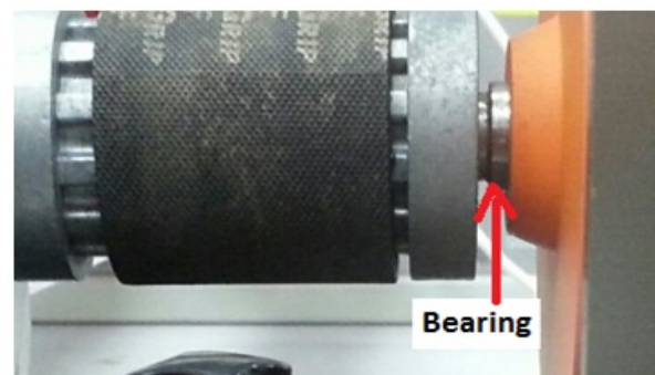
Figure-2. Bearing of three phase induction motor.
