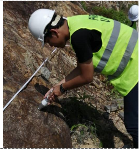
Figure 3. Close up of measurement using the Schmidt rebound hammer
