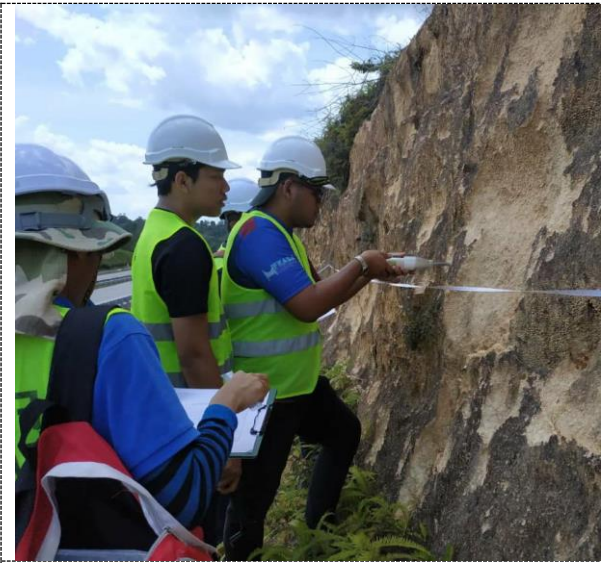
Figure 2. The Schmidt rebound hammer used to identify weathering grade along the scanline of the slope
