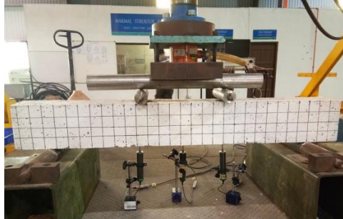
Figure 4. Testing set up for four-points bending test
