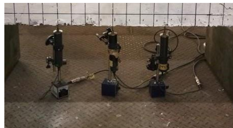
Figure 5. Setup of LVDT under the beam
