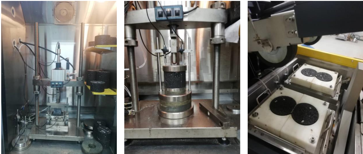
Figure 4. (From left to right) Resilient modulus, dynamic creep and wheel tracking tests
