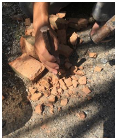
Figure 1. Bricks are crushed using chisel and hammer
