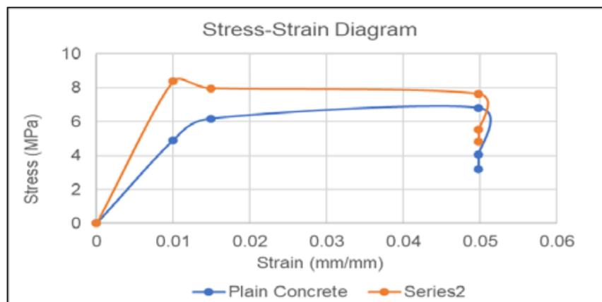
**Figure 6.** Stress-Strain diagram of flexural strength of concrete with 10 mm thickness of the layer.
