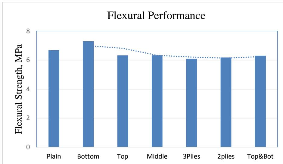
**Figure 3.** Comparison of flexural performance by varied position
