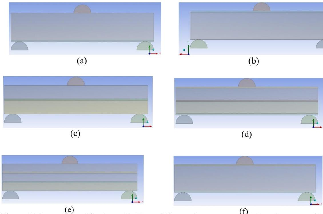
**Figure 1.** The varied position layer thickness of fibrous glass woven as reinforced concrete; (a) Bottom, (b) Top, (c) Middle (d) 3Plies (e) 2Plies (f) Top&Bottom
