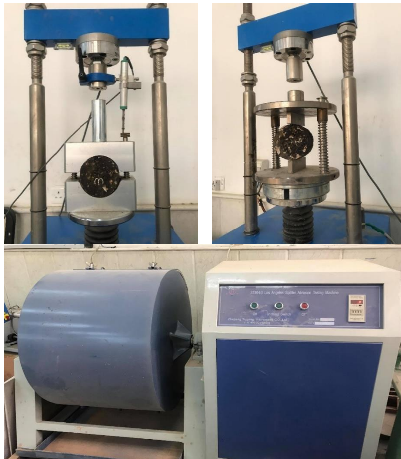
Figure 2. Stability, ITS and Cantabro loss machines
