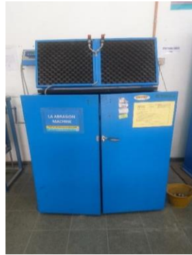
Figure 2. Los Angeles Abrasion Machine
