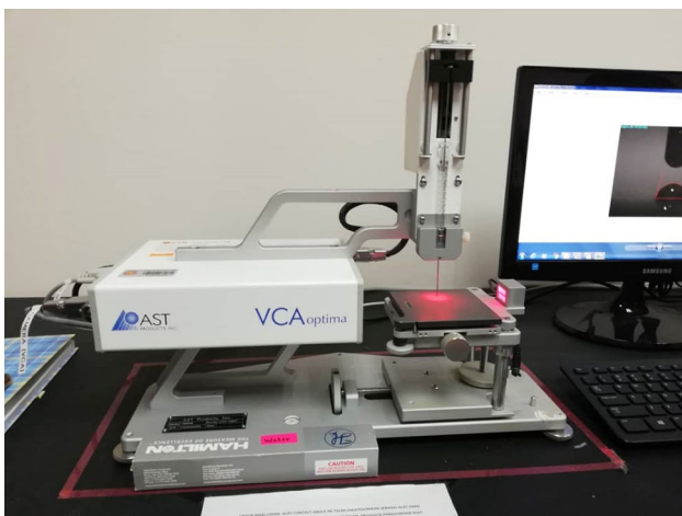
Fig. 3 Contact angle measurements of asphalt surface
