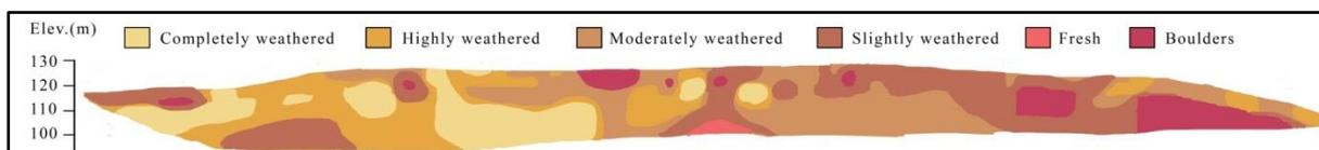
**Figure 5.** Proposed weathering zone for granite of the slope based on electrical resistivity values
