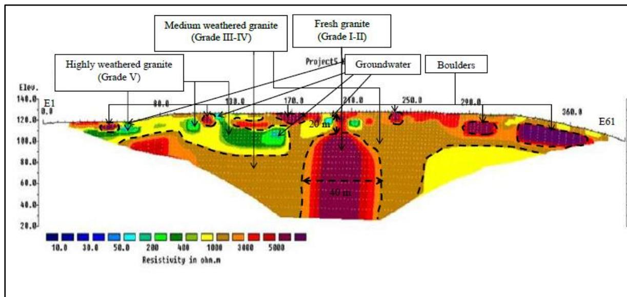
**Figure 3.** Profile of resistivity line, with interpreted weathering zone and groundwater zone
