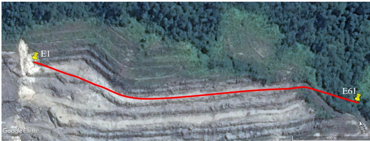
**Figure 1.** Resistivity line of the ERI survey
