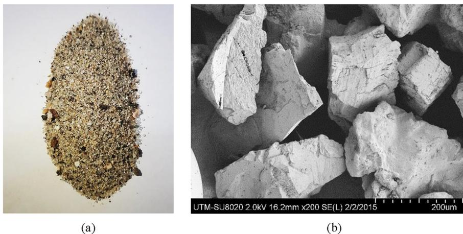
**Fig. 2.** Images of clogging materials (a) raw sample and (b) FESEM image.
