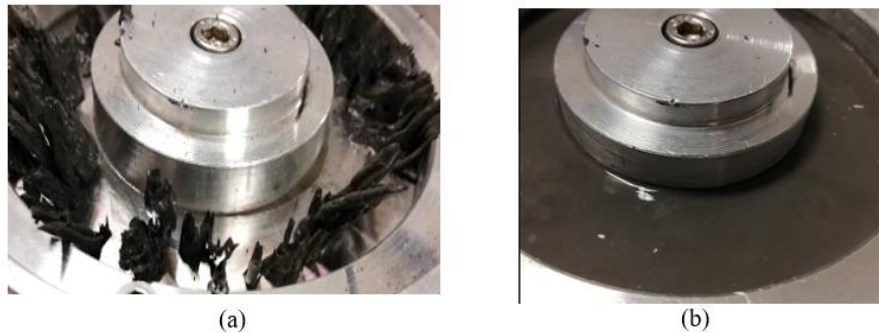
Figure 2: MR fluid (a) with the presence of a magnetic field and (b) without the presence of magnetic field.
