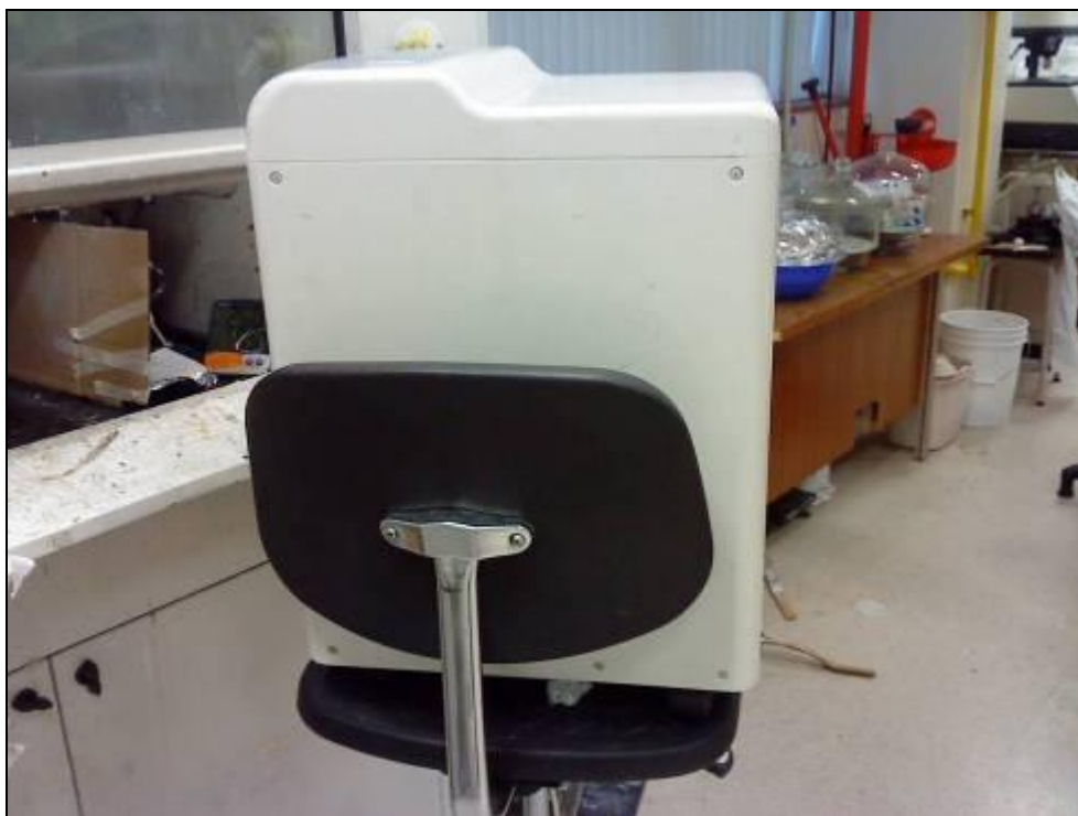
Figure 3.6: Humidifier to control the humidity inside the electrospinning chamber
