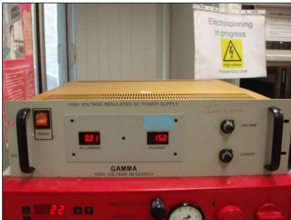
Figure 3.5: High voltage power generator to supply positive direct current to the electrospinning setup
