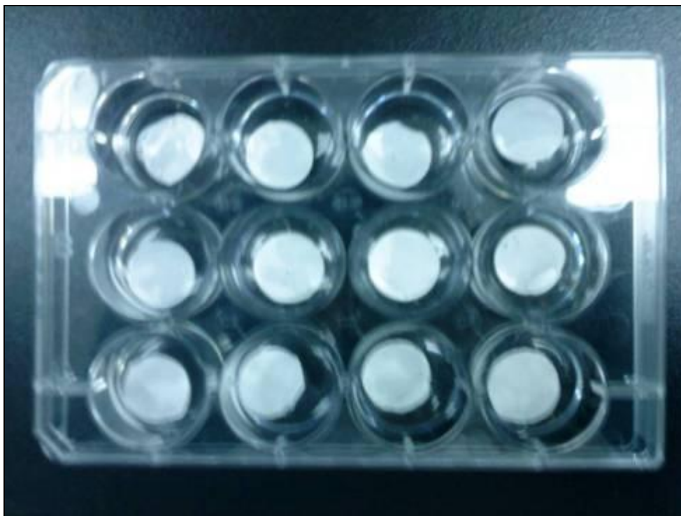
Figure 3.14: PLLACL electrospun nanofibers with proteins mixture loading immersed with 2 mL PBS solution before 24 hours incubation
