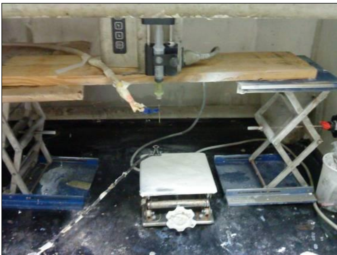
Figure 3.2: Monoxial electrospinning setup. The coaxial electrospinning setup is developed by improvising the above setup using a device designed for coaxial electrospinning purpose
