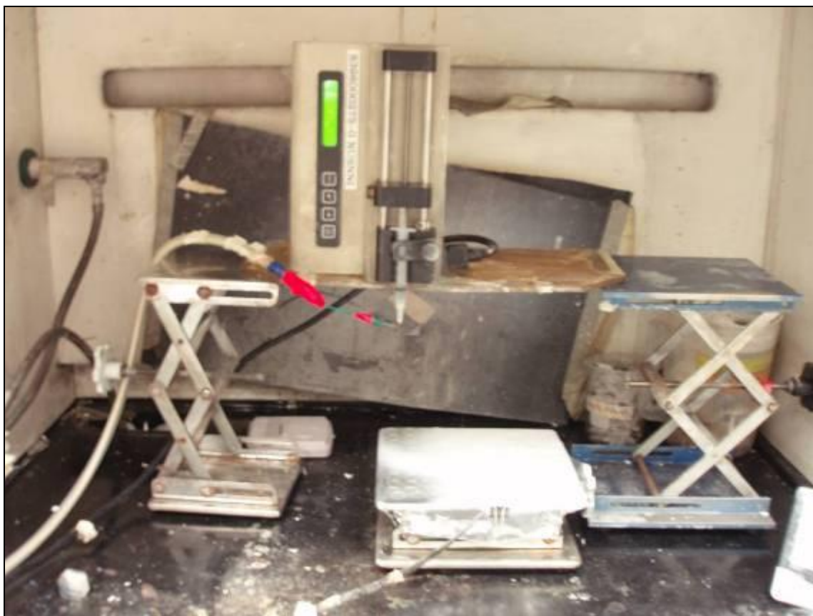
Figure 3.4: Basic electrospinning setup consisting of three major components- a high voltage power supply, a metallic needle (spinneret) and a grounded collector
