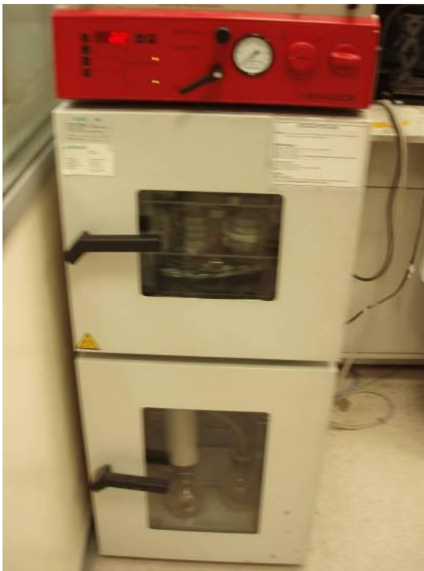
Figure 3.7: Vacuum oven to store the electrospun nanofibers overnight at room temperature
