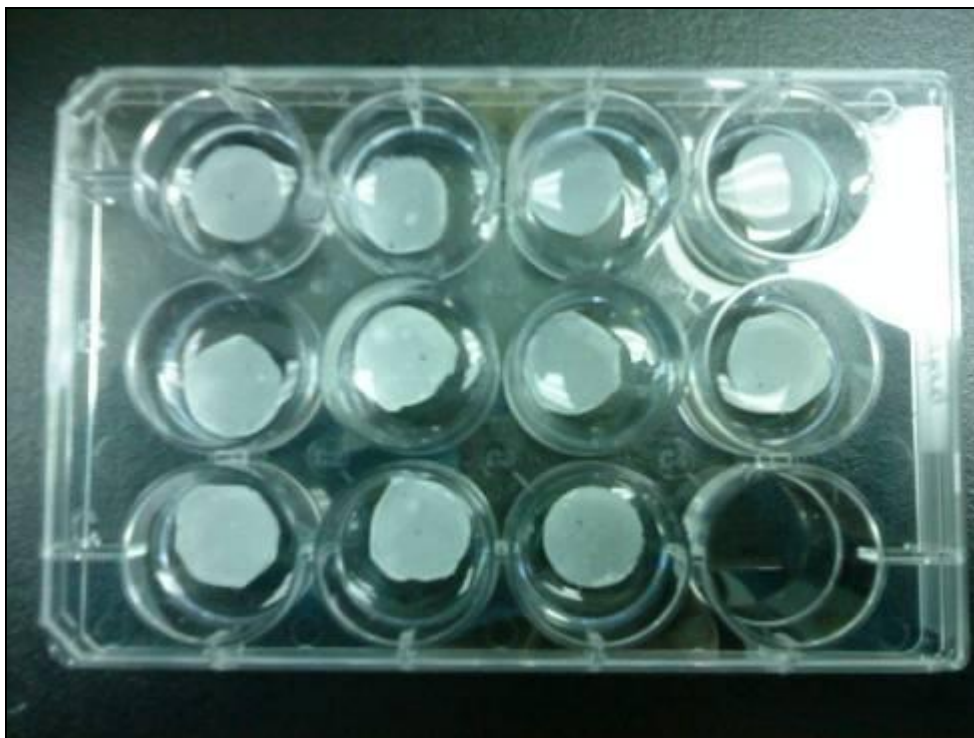
Figure 3.12: PCL electrospun nanofibers with proteins mixture loading immersed with 2 mL PBS solution before 24 hours incubation
