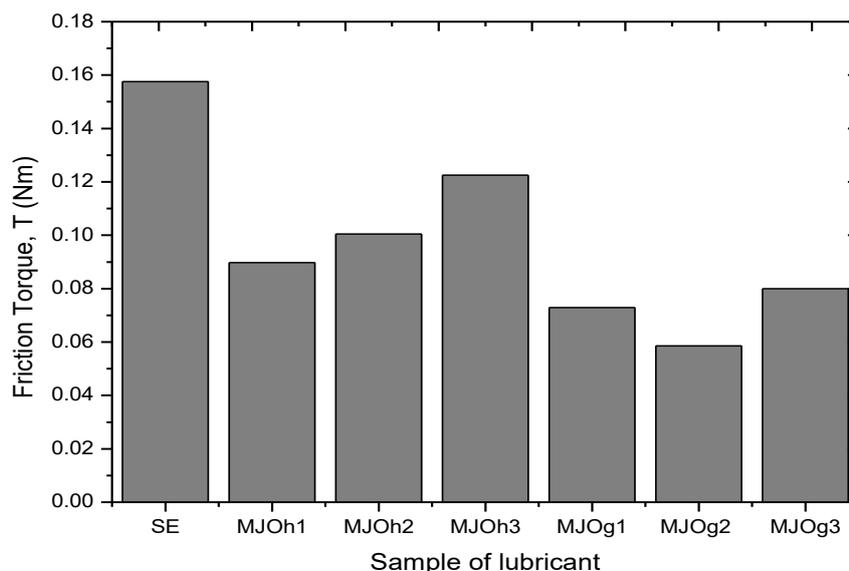
Fig. 7. Variation friction torque of lubricant sample
