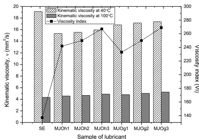
**Fig. 3.** Variation of kinematic viscosity and viscosity index of lubricant sample
