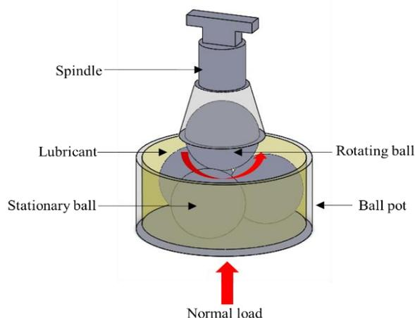
**Fig. 2.** Schematic diagram for four-ball tribo tester
