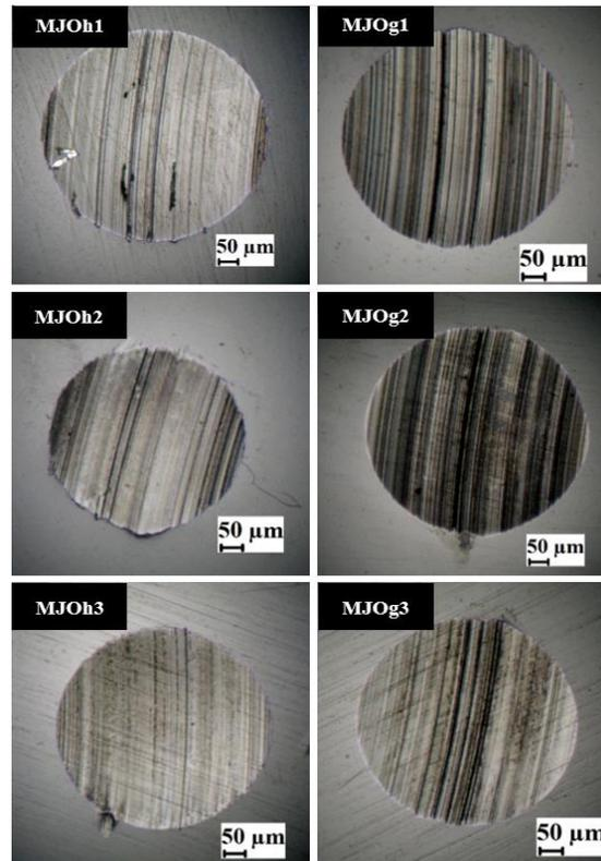
**Fig. 6.** Worn surface of lubricant sample using optical microscope at magnification 5x
