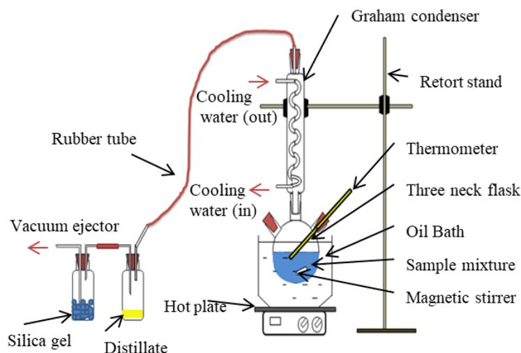
**Fig. 1.** Setup for chemical modification process
