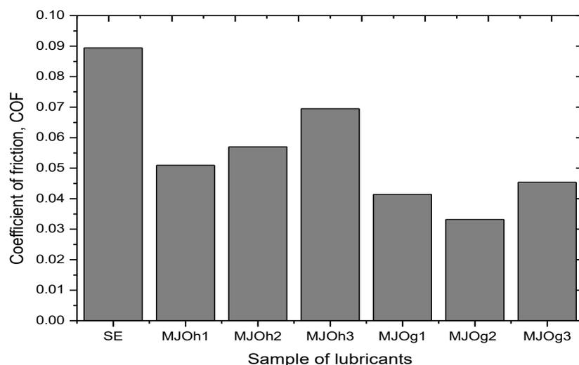
**Fig. 4.** Variation of coefficient of friction for lubricant sample
