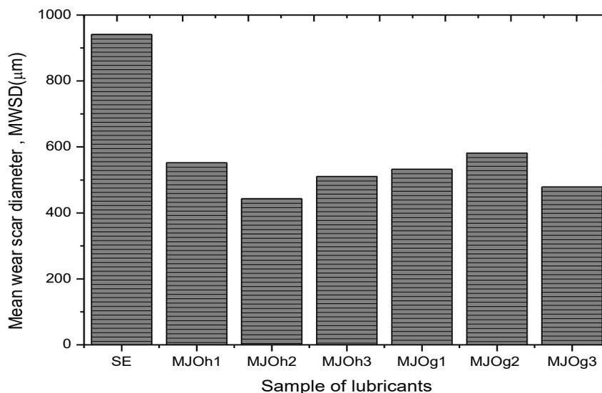
**Fig. 5.** Variation of mean wear scar diameter of lubricant sample
